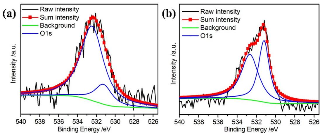
Figure S5 O 1s core-level and corresponding deconvoluted spectra for (a) g-MoSe<sub>2</sub> and (b) g-WSe<sub>2</sub> composite.
