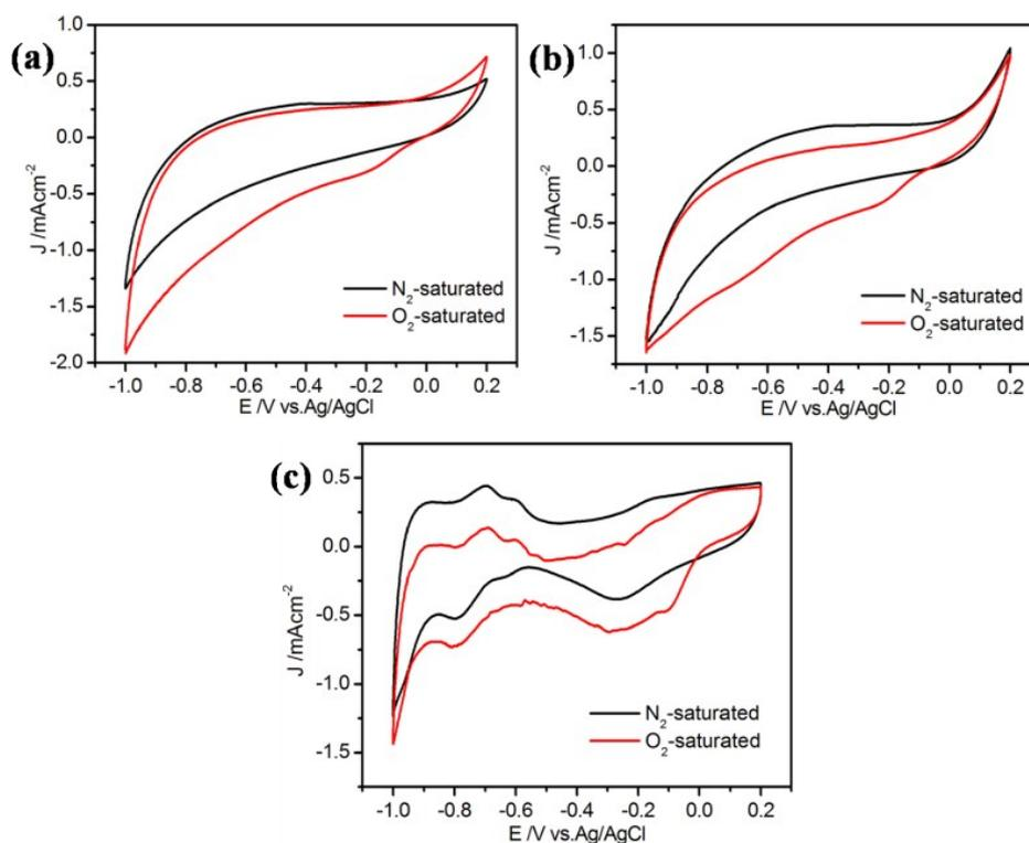
**Figure S7** CVs of (a) MoSe<sub>2</sub>, (b) WSe<sub>2</sub>, (c) Pt/C in N<sub>2</sub>- and O<sub>2</sub>-saturated 0.1M KOH solution at a scan rate of 10 mVs<sup>-1</sup>.
