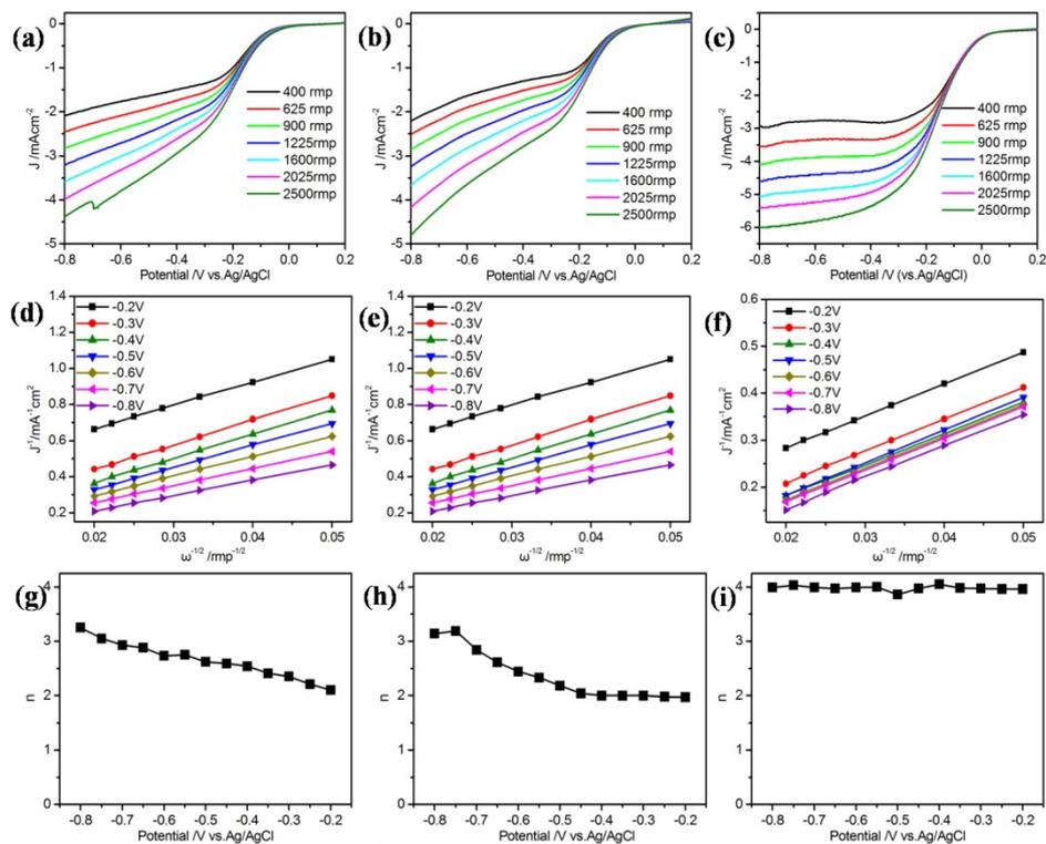
**Figure S8** LSVs of (a) MoSe<sub>2</sub>, (b) WSe<sub>2</sub>, (c) Pt/C in O<sub>2</sub>-saturated 0.1M KOH at a scan rate of 10 mVs<sup>-1</sup> at different RDE rotation rates; The calculated K-L plots of the ORR from (d) MoSe<sub>2</sub>, (e) WSe<sub>2</sub>, (f) Pt/C ; Electron- transfer number *n* (g) MoSe<sub>2</sub>, (h) WSe<sub>2</sub>, (i) Pt/C derived from K–L plots at different potentials.
