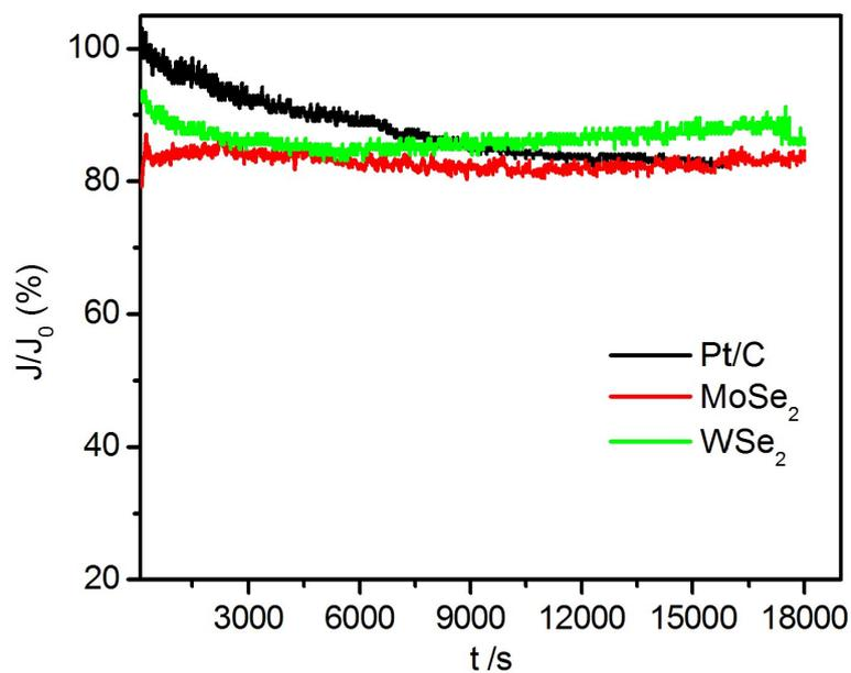
**Figure S9** Chronoamperometric response (*i* – *t*) of MoSe<sub>2</sub> and WSe<sub>2</sub>. The tests were conducted in O<sub>2</sub>-saturated 0.1 M KOH solution at –0.3V.
