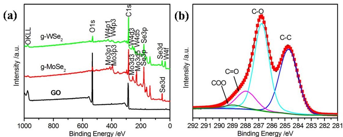
**Figure S6** (a) The survey XPS spectra of g-MoSe<sub>2</sub>, g-WSe<sub>2</sub> and GO, (b) C 1s core-level and corresponding deconvoluted spectra for GO.
