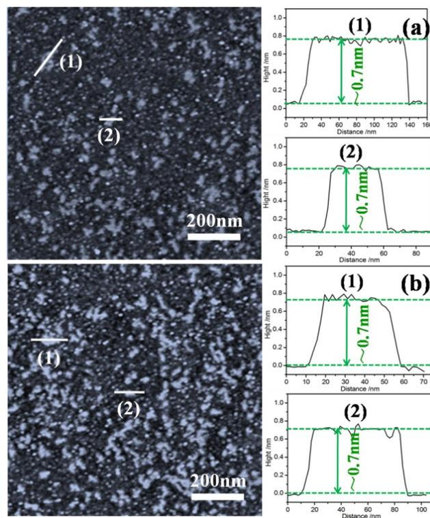
**Figure S3** AFM image and height profiles from sections as indicated by the white lines of MoSe<sub>2</sub> (a) and WSe<sub>2</sub> (b).
