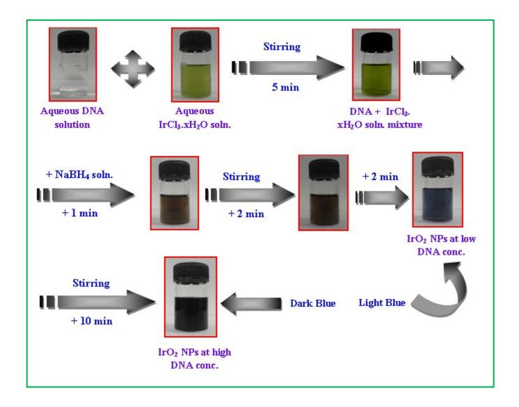
Scheme S1: The schematic depiction of the overall preparation process for the formation of self-assembled  $DNA@IrO_2 NPs$ .
