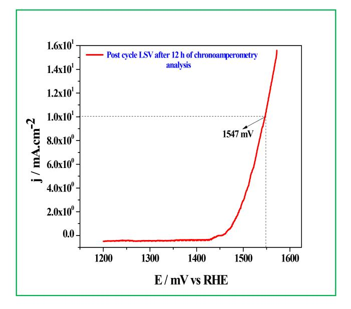
**Figure S2:** iR corrected linear sweep voltammogram of DNA-IrO<sub>2</sub> NPs modified GC after the chronoamperometry analysis at a sweep rate of  $0.01 \text{ V.s}^{-1}$ .
