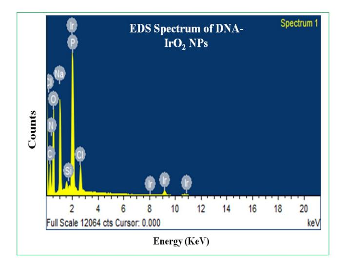
**Figure S1:** The energy dispersive X-ray spectroscopic (EDS) analysis of self-assembled IrO<sub>2</sub> NPs on DNA scaffold that possess the expected peaks for Ir, Cl, O, Ca, Si, P and Na.
