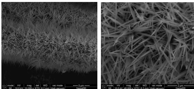
**Figure S1.** SEM images of  $\text{Co(OH)}_2$  nanowires on CC.
