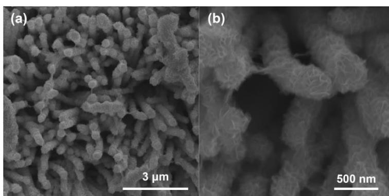
**Figure S3.** SEM images of  $\text{MoS}_2/\text{CoS}_2/\text{CC}$  after i-t testing.
