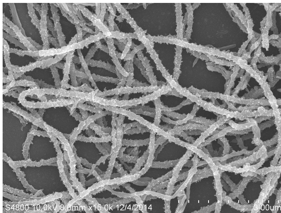
Fig. S3 FESEM image of PEDOT nanofibres after being dispersed.
