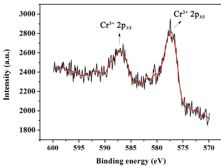
**Fig. S18** XPS spectrum of  $\text{Cr}^{3+}$  for  $\text{Cr}^{3+}$ @NENU-505.
