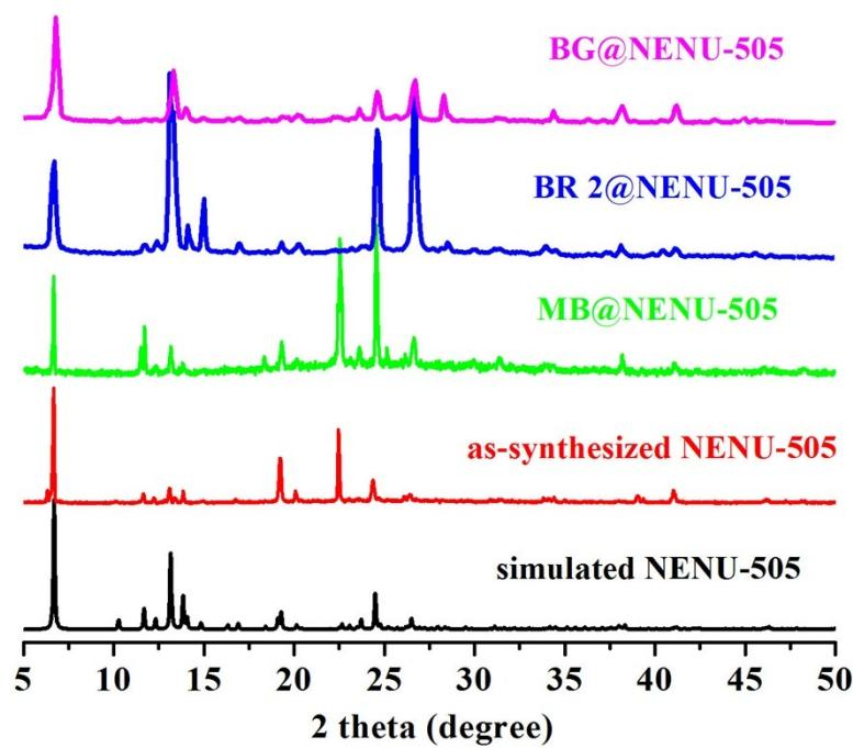
**Fig. S6** XRPD patterns of simulated NENU-505 (black), as-synthesized NENU-505 (red) and after the absorption of MB (green), BR 2 (blue) and BG (pink), respectively.
