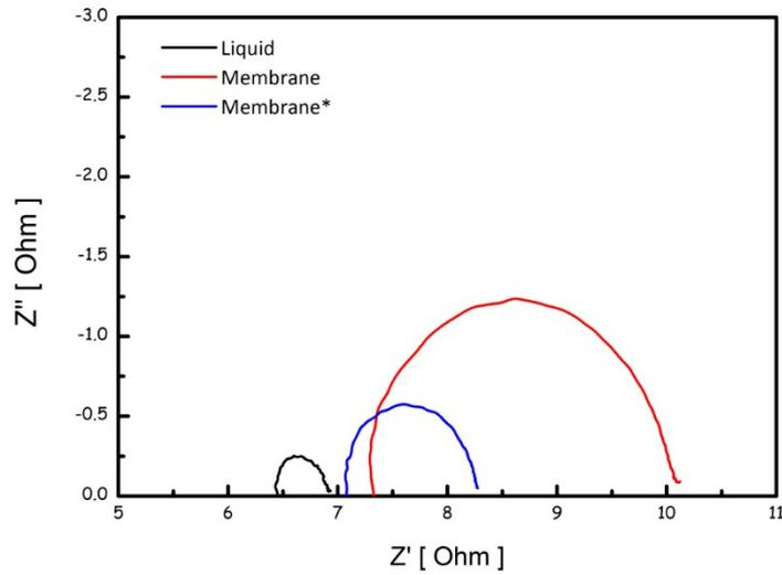
**Figure S2. Electrolyte bulk resistance under the frequency range of 0.1 Hz to 100 kHz and AC oscillation of 10 mV**
