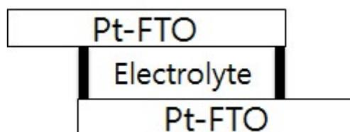
**Figure S1. The symmetrical cell used for the measurements**
