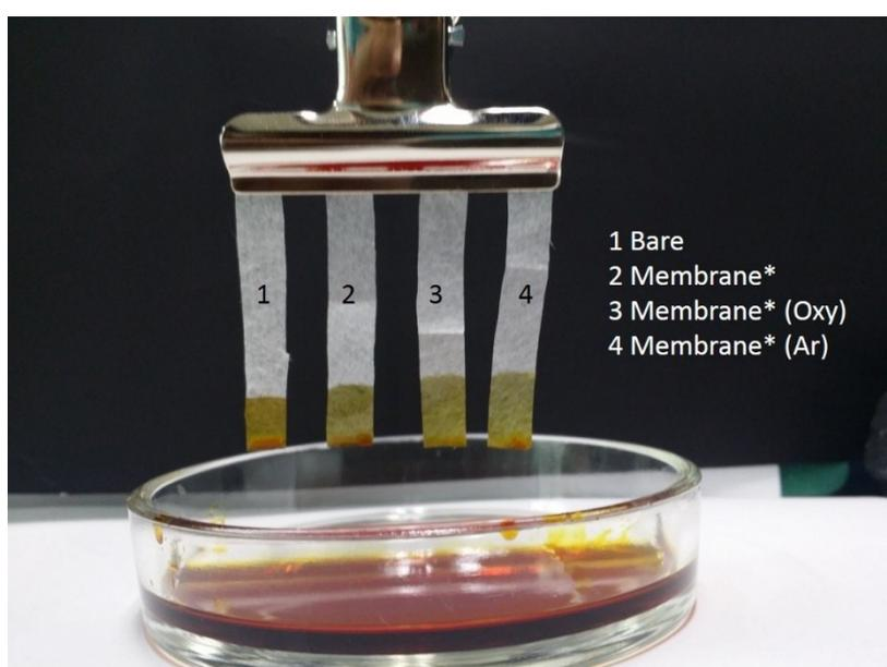
**Figure S5. Wicking test analysis of nonwoven PET membrane in electrolyte**
