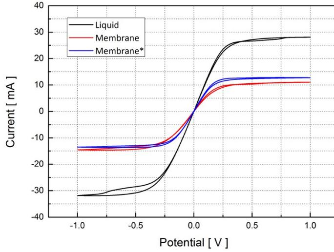
**Figure S3. Steady-state current-potential curve of the symmetrical cells using different electrolyte**
