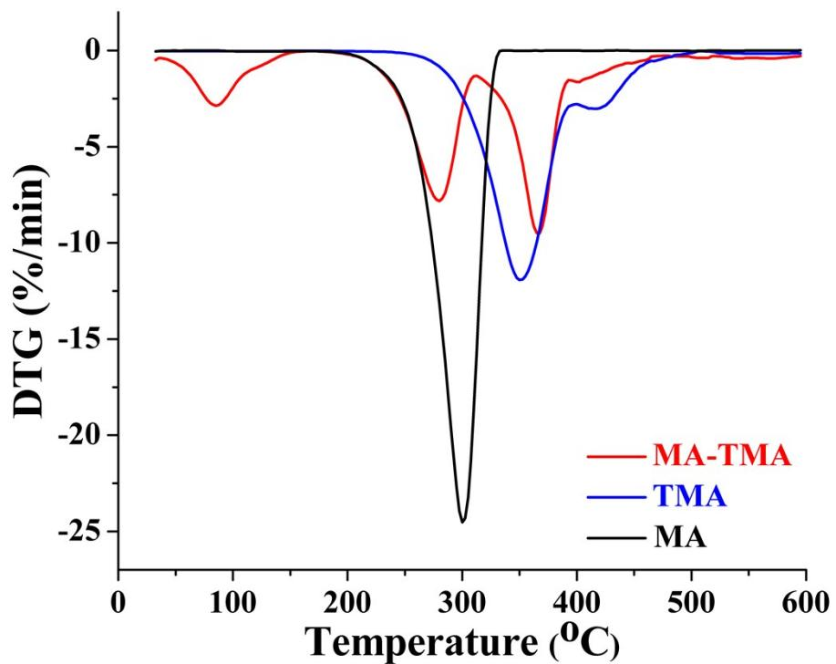
Fig. S3 DTG analysis of MA, TMA, and MA-TMA.
