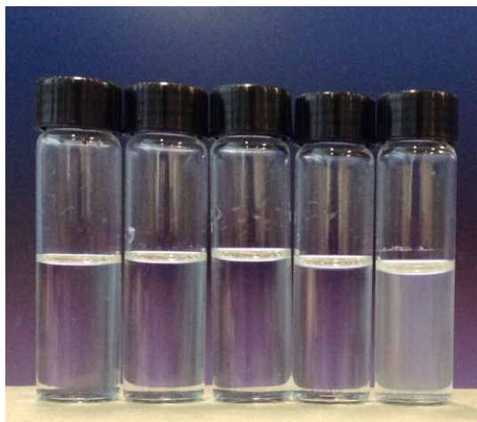
Figure SI-1. Stability characteristics of the hydroxo-aquo ions of titanium precursors in high acidic solution (6 M HCl). The five bottles from left to right contain the solutions hydrothermally treated at room temperature, 50 °C, 80 °C, 100 °C, and 120 °C for 6 hours, respectively. In this photograph, it is clear to see that titanium precursors are stable in acidic solution at low temperature (< 100 °C); while they become unstable once temperature increases (> 100 °C).
