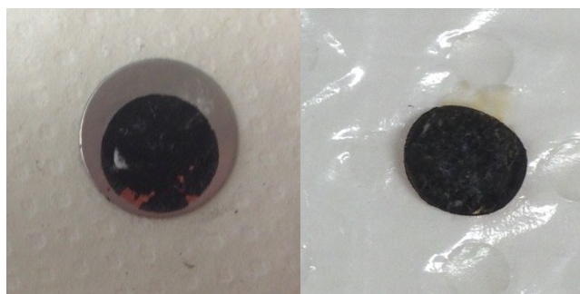
Figure S10. Photographs of the electrodes after 200 cycles: (a) P/GnPs-300; (b) P/GnPs -500.
