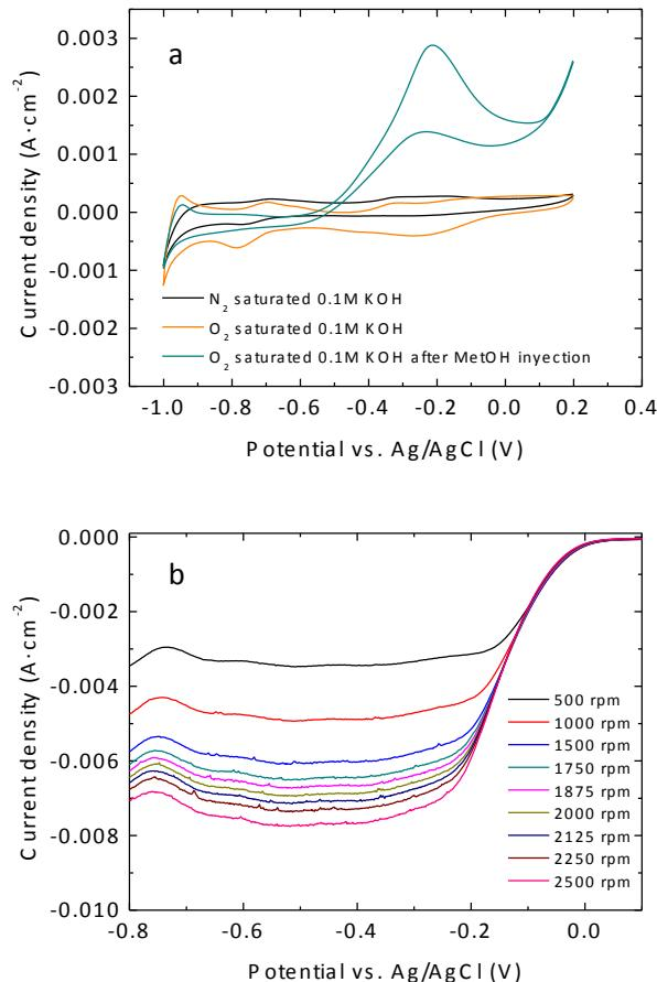
**Figure S7** – CV recorded after stability test (blue line) and at 1600 rpm of R4CPC carbon in  $N_2$  saturated 0.1 M KOH (black line), in  $O_2$  saturated 0.1 M KOH (red line) and in  $O_2$  saturated 0.1 M KOH.
