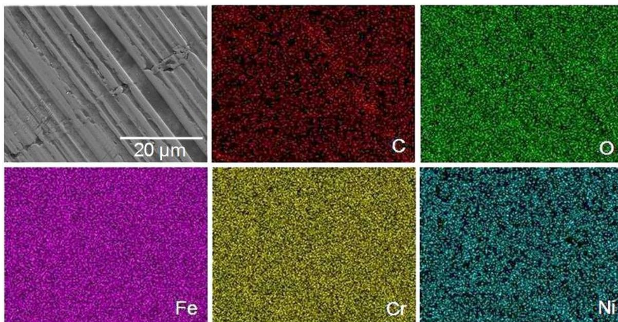
**Figure S7.** FESEM micrograph and corresponding element mapping images on the worn track of steel disc lubricated with PEG 200 lube base oil. Load: 2 N, speed: 1 cm.s<sup>-1</sup>, sliding distance: 100 meter.
