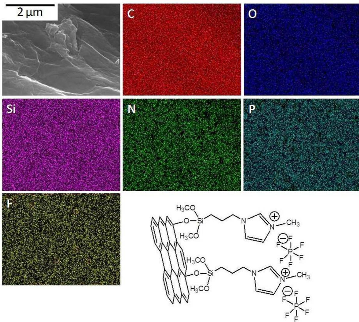
**Figure S4.** FESEM micrograph and corresponding element mapping images of Gr-PF<sub>6</sub> hybrid nanomaterial along with its representative molecular structure. The element symbol is mentioned on each image.
