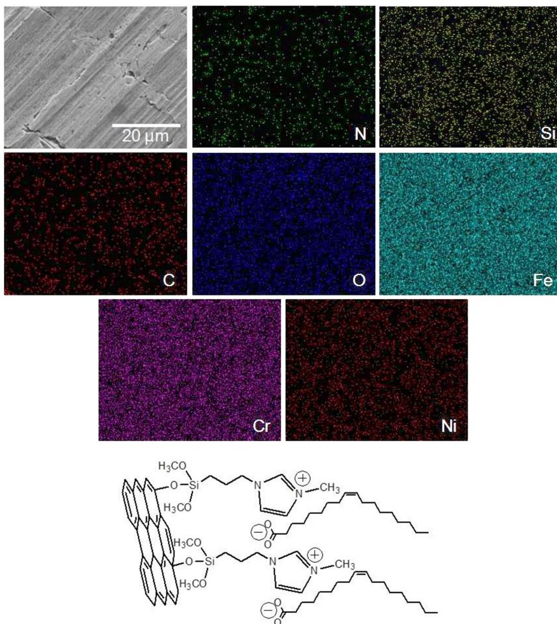
**Figure S8.** FESEM micrograph and corresponding element mapping images on the worn track of steel disc lubricated with Gr-OL blended with PEG 200 lube base oil (dose:  $0.02 \text{ mg}\cdot\text{mL}^{-1}$ ). The uniform distribution of nitrogen and silicon on the worn track of steel disc revealed the contribution of Gr-OL hybrid nanomaterial in formation of tribo-thin film, which reduces the friction and wear. The representative molecular structure of Gr-OL is shown separately.
