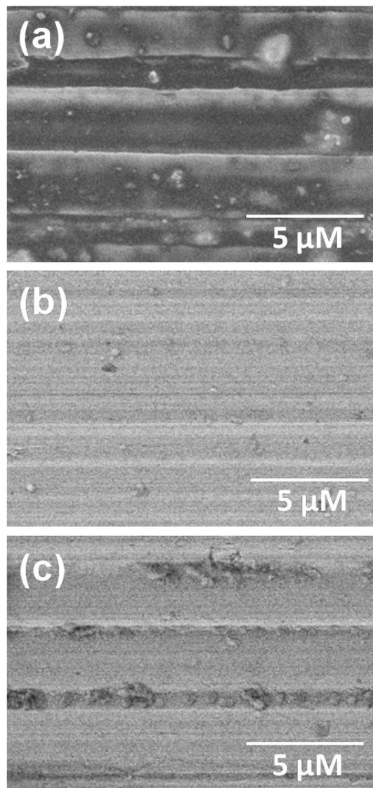
**Figure S5:** FESEM micrograph images of worn track of steel disc lubricated with (a) PEG and variable dose of Gr-BScB (b) 0.02 and (c) 0.05 mg.mL<sup>-1</sup> blended samples.
