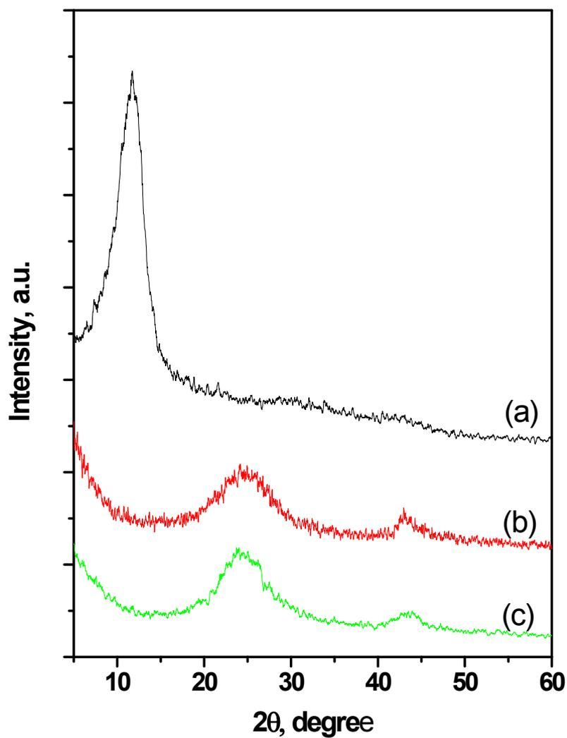
**Figure S1:** XRD patterns of (a) GO, (b) rGO, prepared by chemical reduction of GO. (c) Carboxylic group enriched graphene nanosheets, prepared by mild oxidation of rGO. XRD patterns reveals that during mild oxidation of rGO, the graphene characteristic interlayer distance remains intact.
