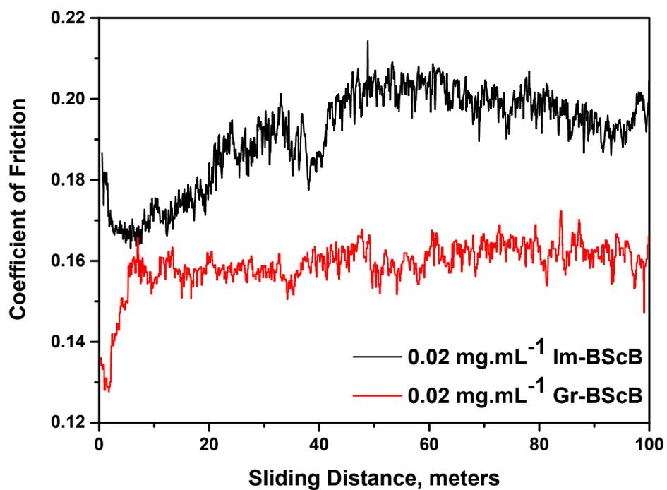
**Figure S6:** Changes in coefficient of friction as a function of individual blends of Im-BScB ionic liquid and Gr-BScB hybrid nanomaterial in PEG 200 (0.02 mg.mL<sup>-1</sup>) under reciprocating sliding contact of steel tribo-pair. Load: 2 N, speed: 3 cm.s<sup>-1</sup>, mean Hertzian contact pressure: 810 MPa
