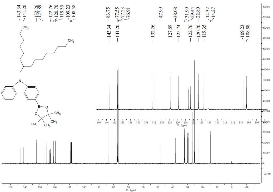
**Fig. S11** The  $^{13}\text{C}$  NMR (100 MHz) of **8** in  $\text{CDCl}_3$ .
