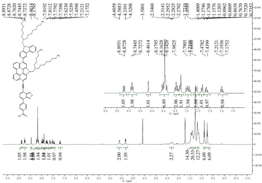
**Fig. S18** The  $^1\text{H}$  NMR (400 MHz) of HW-3 in THF.
