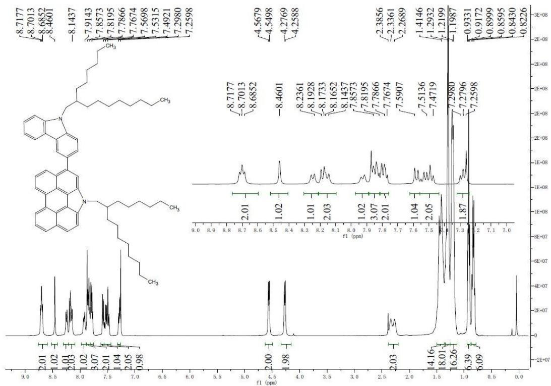
**Fig. S12** The  $^1\text{H}$  NMR (400 MHz) of **2** in  $\text{CDCl}_3$ .
