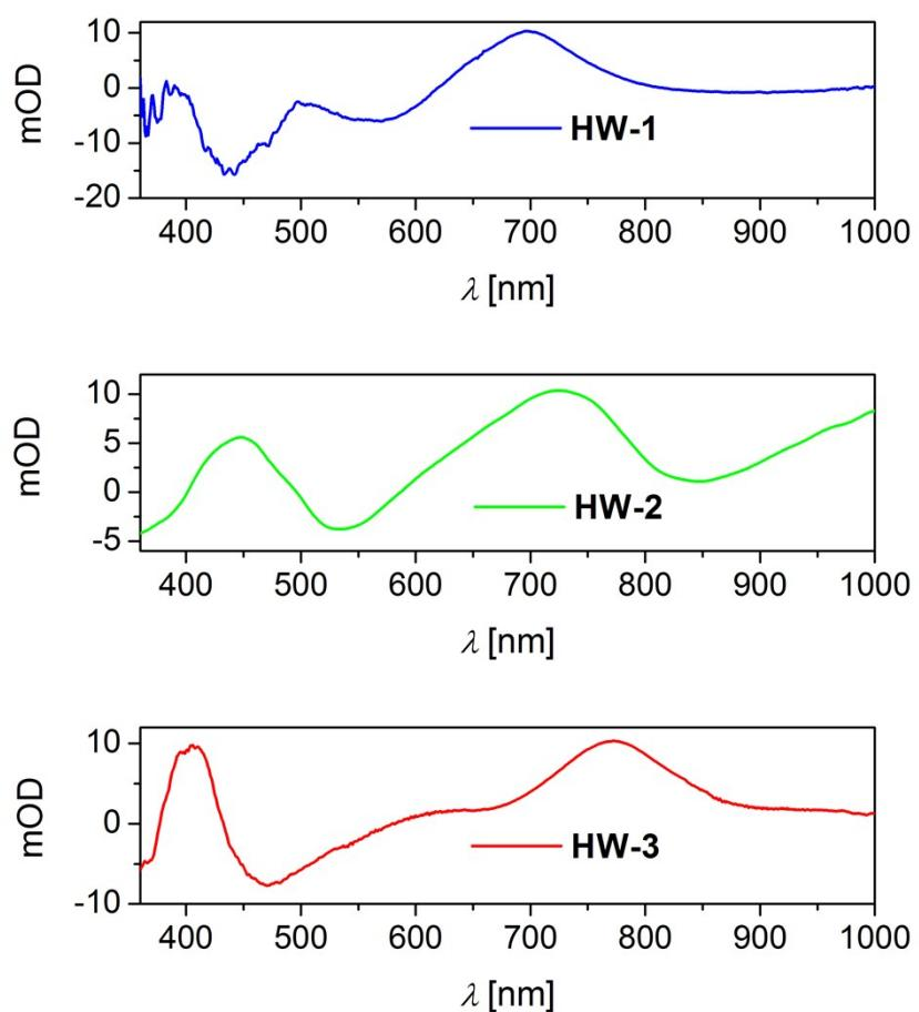
**Fig. S1** Wavelength-dependent absorption change upon applying a positive potential bias to a 1.2- $\mu\text{m}$ -thick, dye-grafted titania film immersed in EMITFSI.
