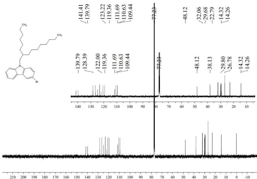
**Fig. S9** The  $^{13}\text{C}$  NMR (100 MHz) of 7 in  $\text{CDCl}_3$ .
