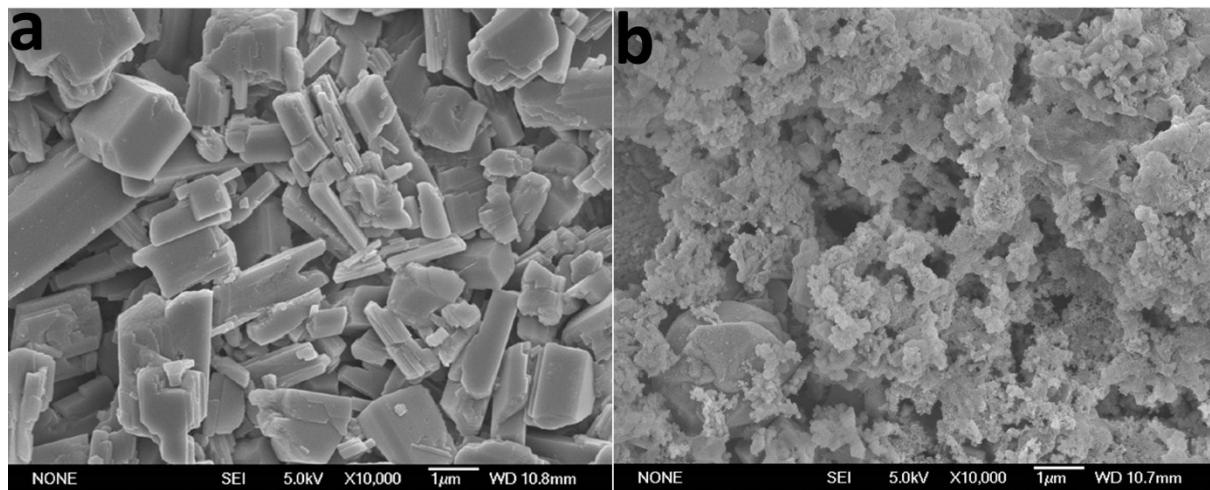
Figure S3: SEM images of the products after reaction of mill scale with (a) oxalic acid and (b) HCl.
