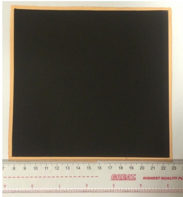
Figure S8: Photograph of a 15 cm x 15 cm sprayed electrode on a Cu foil current collector
