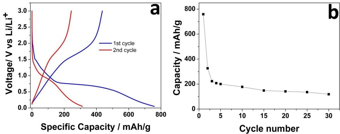
Figure S7: (a) Charge/discharge curves at 0.1 C of the ball milled mill scale powder and (b) specific capacity as a function of cycle number.
