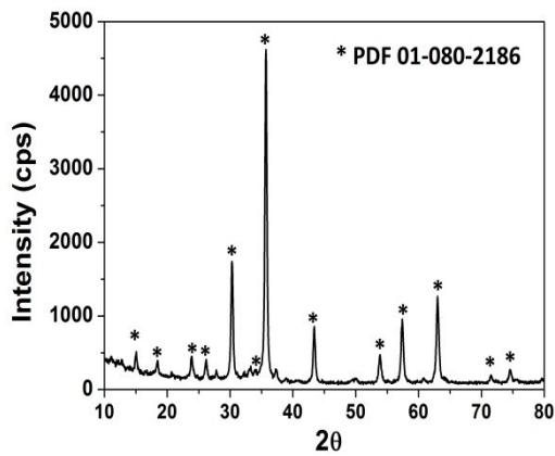
Figure S4: XRD pattern of the product obtained after calcination at 400 °C for 2 hrs.
