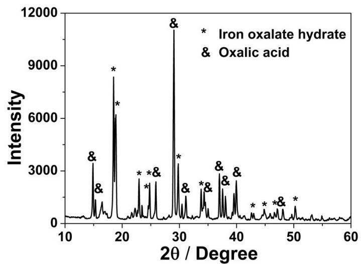
Figure S2: XRD pattern of the product after reaction of the mill scale with oxalic acid.
