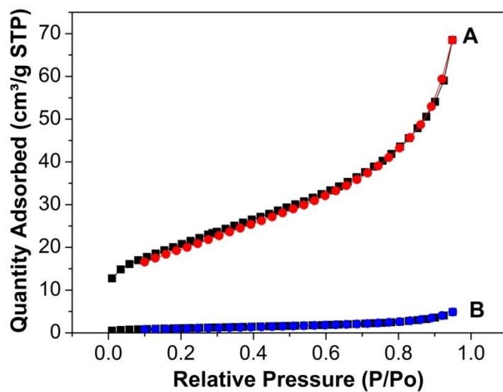
Figure S6:  $\text{N}_2$  adsorption-desorption isotherms of the feedstock mill scale powder after 4 hr ball milling (B) and then the hollow and porous  $\text{Fe}_2\text{O}_3$  powder after chemical and heat treatment (A).
