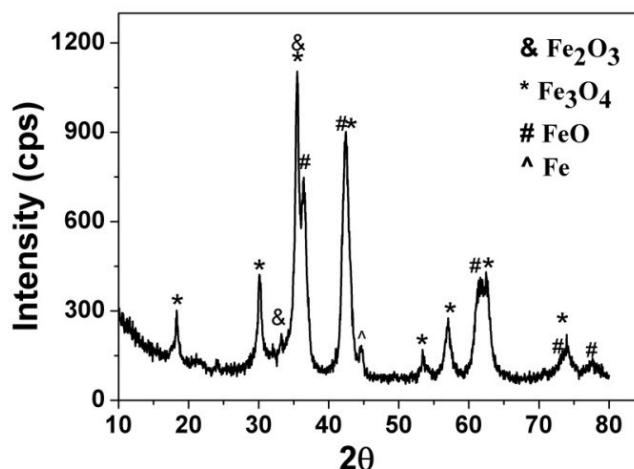
Figure S1: XRD pattern of the as-supplied mill scale
