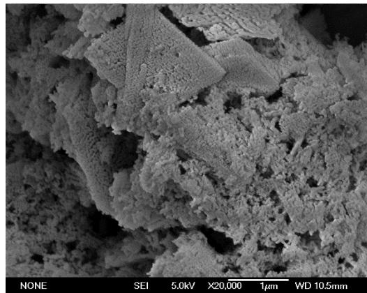
Figure S5: SEM image of the product obtained after calcination at 800 °C for 2 hrs.
