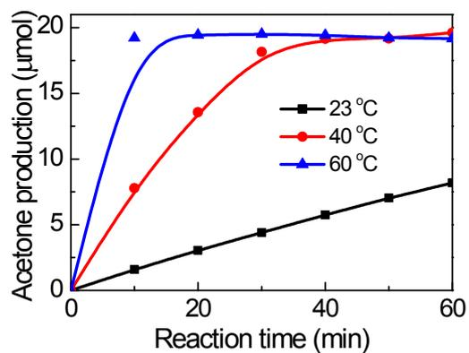
Fig. S6 Catalytic performance of Au/SrTiO<sub>3</sub>-urea catalyst in IPA dehydrogenation at different reaction temperatures.
