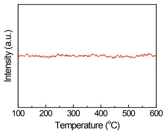
Fig. S9 O<sub>2</sub>-TPD profile of Au/SrTiO<sub>3</sub>-urea catalyst.
