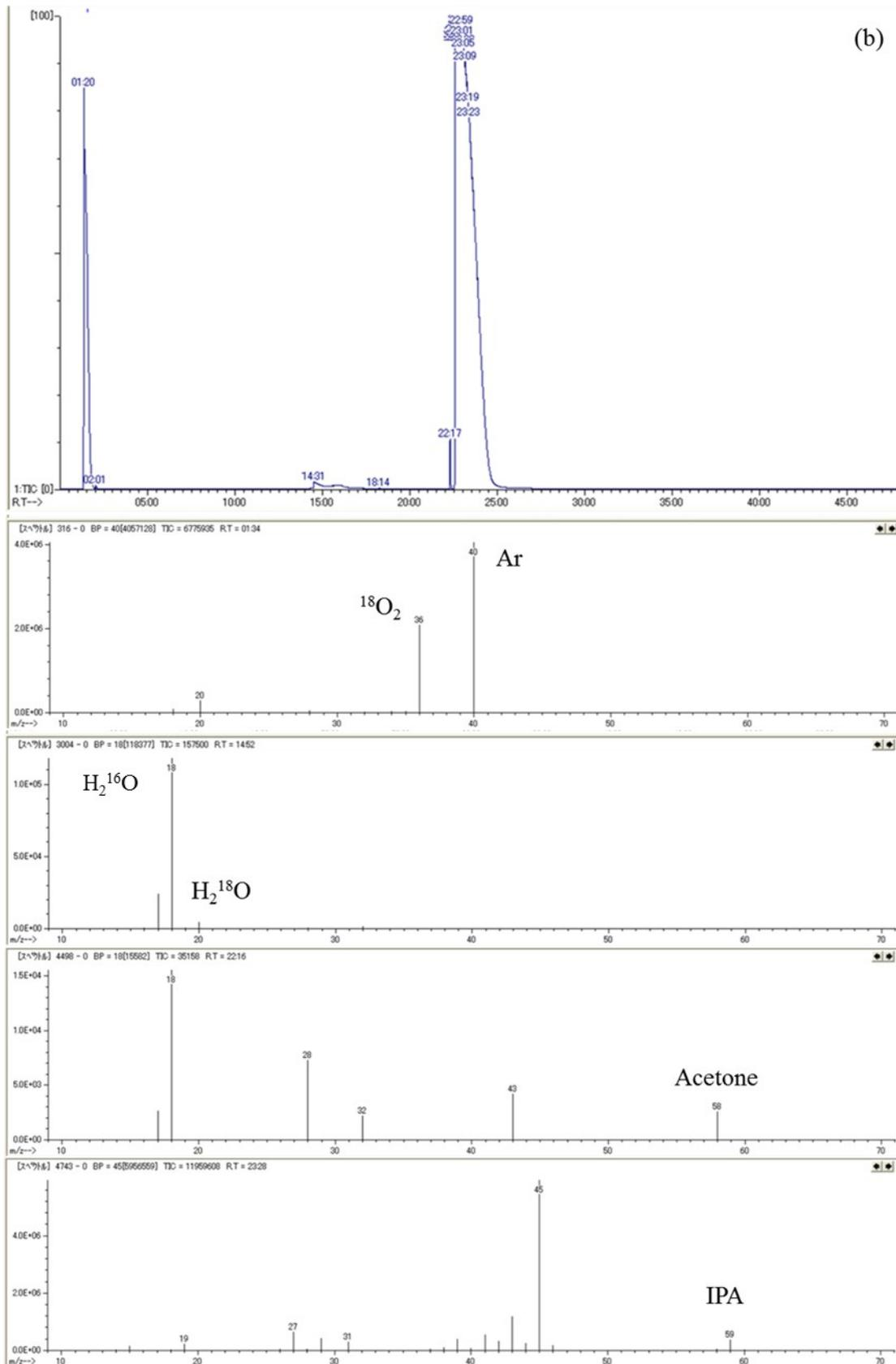
Fig. S8  $^{18}\text{O}_2$  isotope experiment over Au/SrTiO<sub>3</sub>-urea catalyst.
