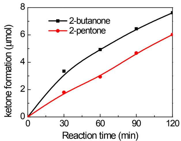
Fig. S12 Catalytic performance of the Au/SrTiO<sub>3</sub>-urea catalyst in 2-butanol and 2-pentanol dehydrogenation.
