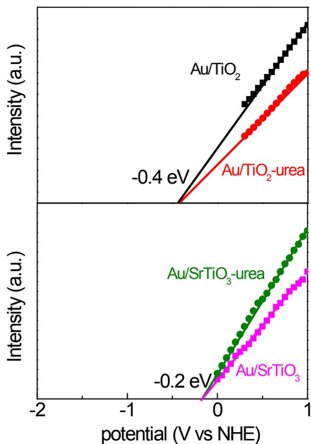
Fig. S13 Mott-Schottky plots of the Au-based catalysts.
