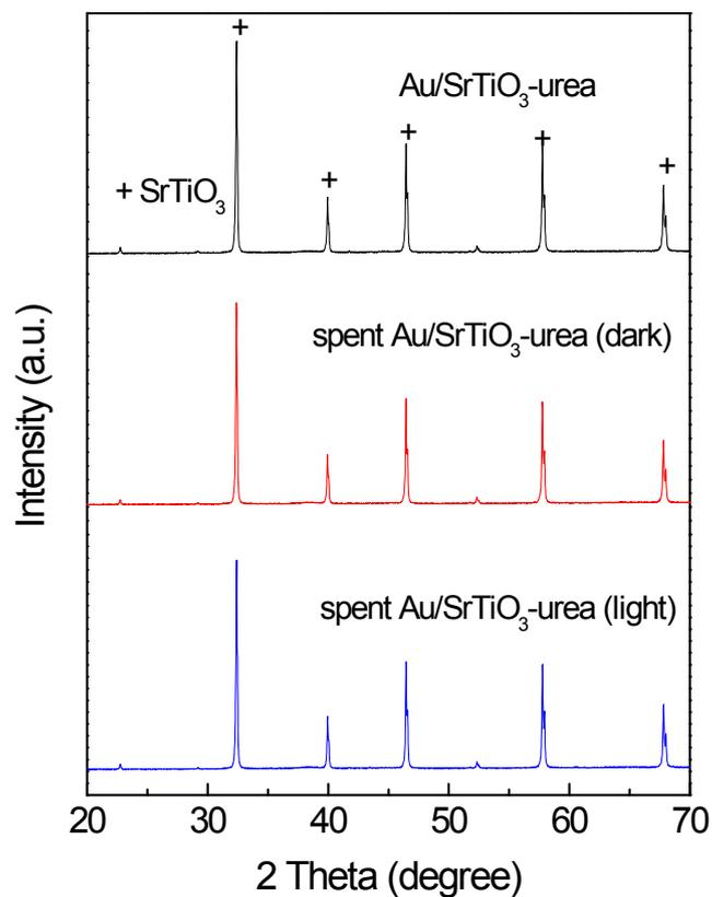
Fig. S15 XRD patterns of the fresh and spent Au/SrTiO<sub>3</sub>-urea catalysts.
