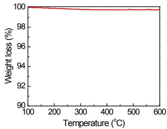
Fig. S10 TGA profile of Au/SrTiO<sub>3</sub>-urea catalyst.
