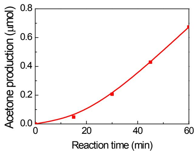
Fig. S5 Catalytic performance of Pt/TiO<sub>2</sub> catalyst in IPA dehydrogenation.
