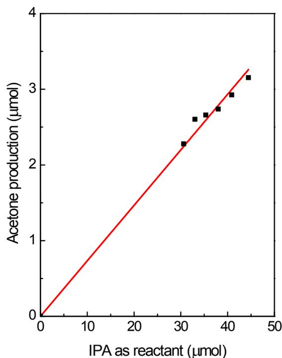
Fig. S4 Relationship between the amount of acetone production in 10 min and the initial IPA concentration at room temperature (23 °C) over Au/SrTiO<sub>3</sub>-urea without light irradiation.
