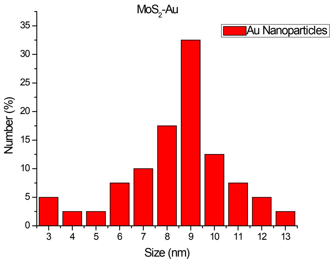
**Fig. S8:** Size distribution of  $\text{MoS}_2\text{-Au}$  assemblies, produced by a single, of  $100\text{mJcm}^{-2}$ , UV pulse.
