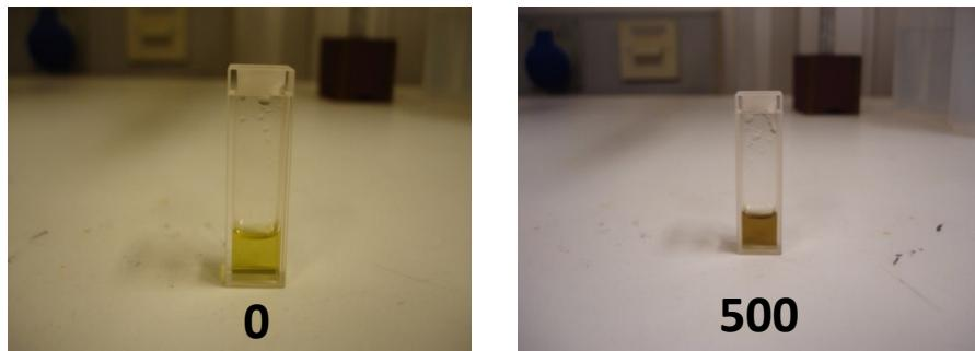
**Fig. S4:** Pictures of the reference and laser treated WS<sub>2</sub>-AgNO<sub>3</sub> dispersions, irradiated with 500, 100mJcm<sup>-2</sup>, UV pulses.
