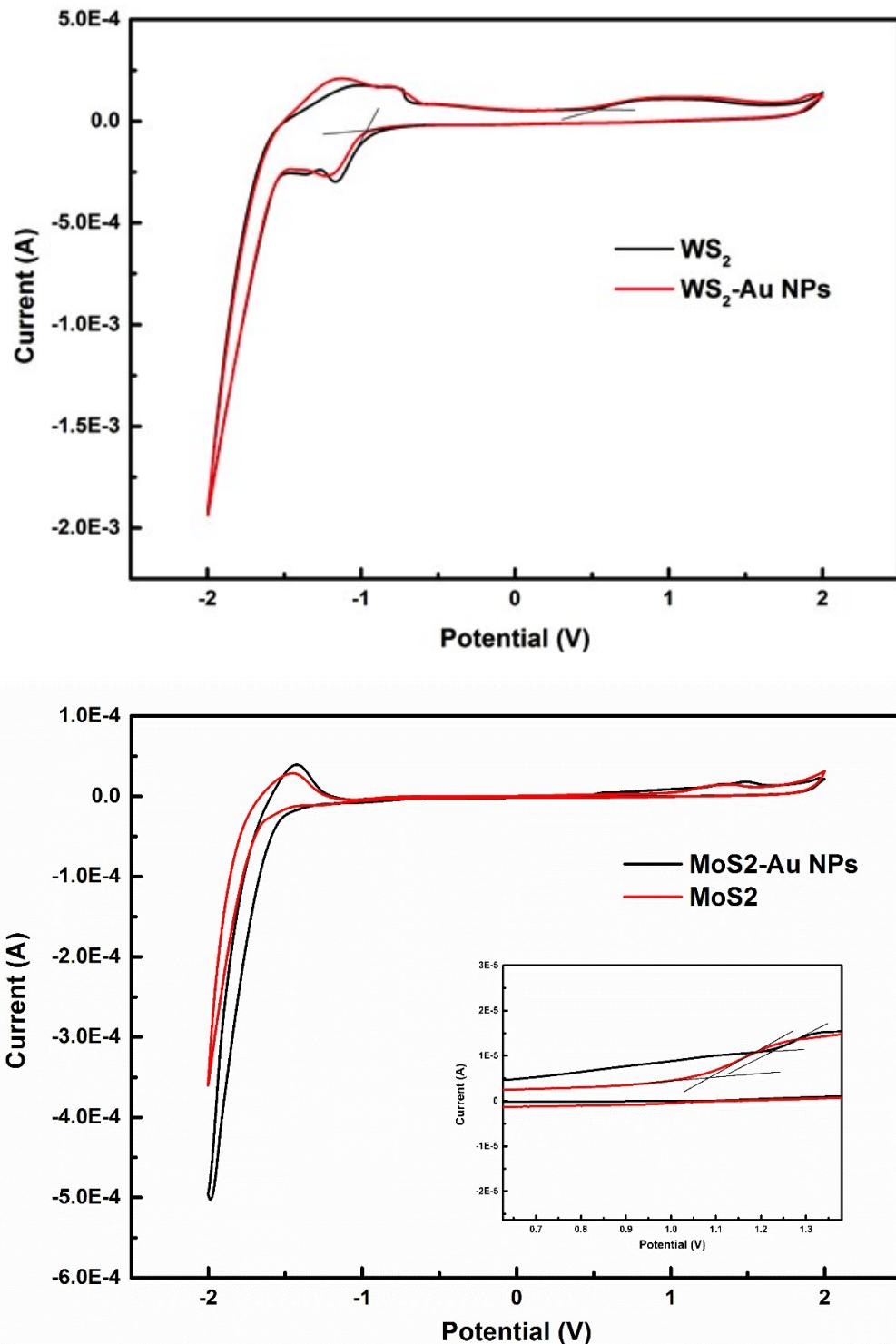
**Fig. S12:** (Top) Cyclic voltammogram of WS<sub>2</sub> and WS<sub>2</sub>-Au NPs in CH<sub>3</sub>CN using 0.1 M TBAPF<sub>6</sub> as electrolyte. Scan rate was set at 100 mV s<sup>-1</sup>. (Bottom) Cyclic voltammogram of MoS<sub>2</sub> and MoS<sub>2</sub>-Au NPs in CH<sub>3</sub>CN using 0.1 M TBAPF<sub>6</sub> as electrolyte. Scan rate was set at 10 mV s<sup>-1</sup>.
