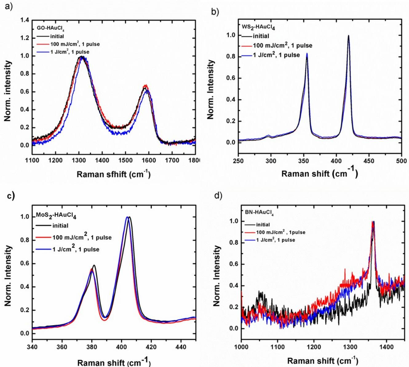
**Figure S11.** Normalized Raman spectra of a) GO, b) WS<sub>2</sub>, c) MoS<sub>2</sub> and d) BN NS before and after laser induced decoration with Au NPs.
