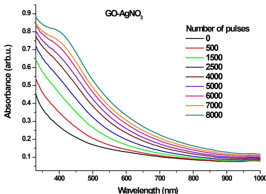
**Fig. S1:** UV-vis absorption spectra of pristine GO-AgNO<sub>3</sub> dispersions in water, irradiated with different numbers of 100mJcm<sup>-2</sup> UV pulses.
