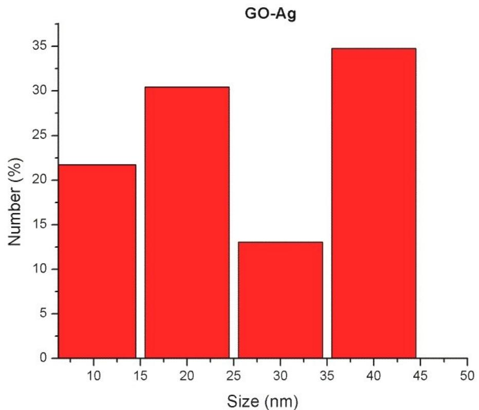
**Fig. S3:** Size distribution GO-Ag assemblies, produced by a single, of  $100\text{mJcm}^{-2}$ , UV pulse.
