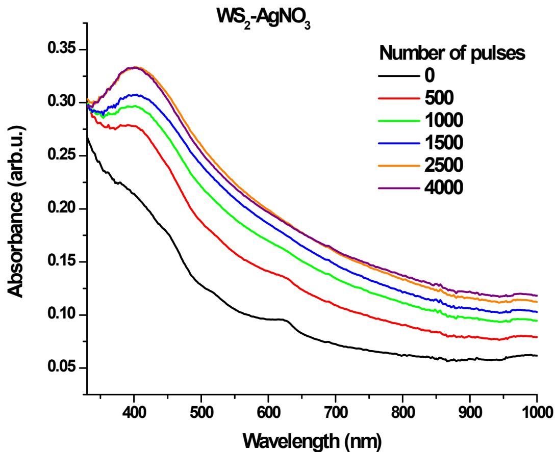
**Fig. S5:** UV-vis absorption spectra of pristine WS<sub>2</sub>-AgNO<sub>3</sub> dispersions in water, irradiated with different numbers of 100mJcm<sup>-2</sup> UV pulses.
