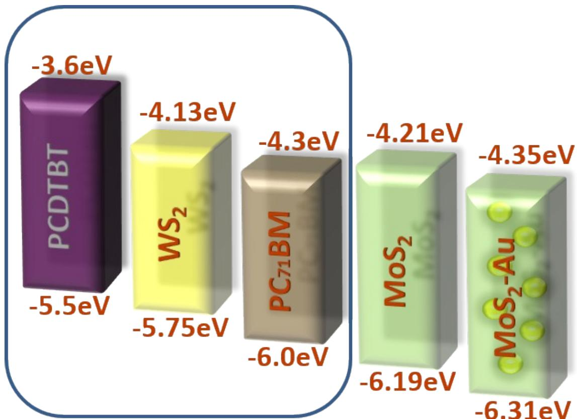
**Figure S16:** Energy level diagram of the materials investigated for ternary OPV devices.
