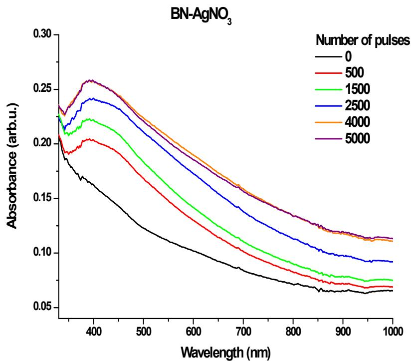
**Fig. S9:** UV\_VIS spectra of BN-AgNO<sub>3</sub> dispersions in water, irradiated with different numbers of 100mJcm<sup>-2</sup> UV pulses.
