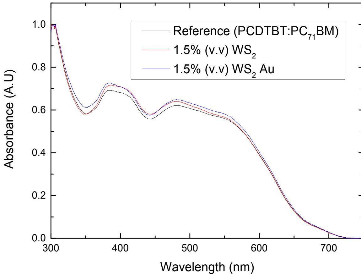
**Fig. S13:** Absorption spectra of PCDTBT:PC71BM (Reference cell), ternary Solar cell with 1.5% (v/v) WS<sub>2</sub> and ternary Solar cell with 1.5% (v/v) WS<sub>2</sub> Au NPs.
