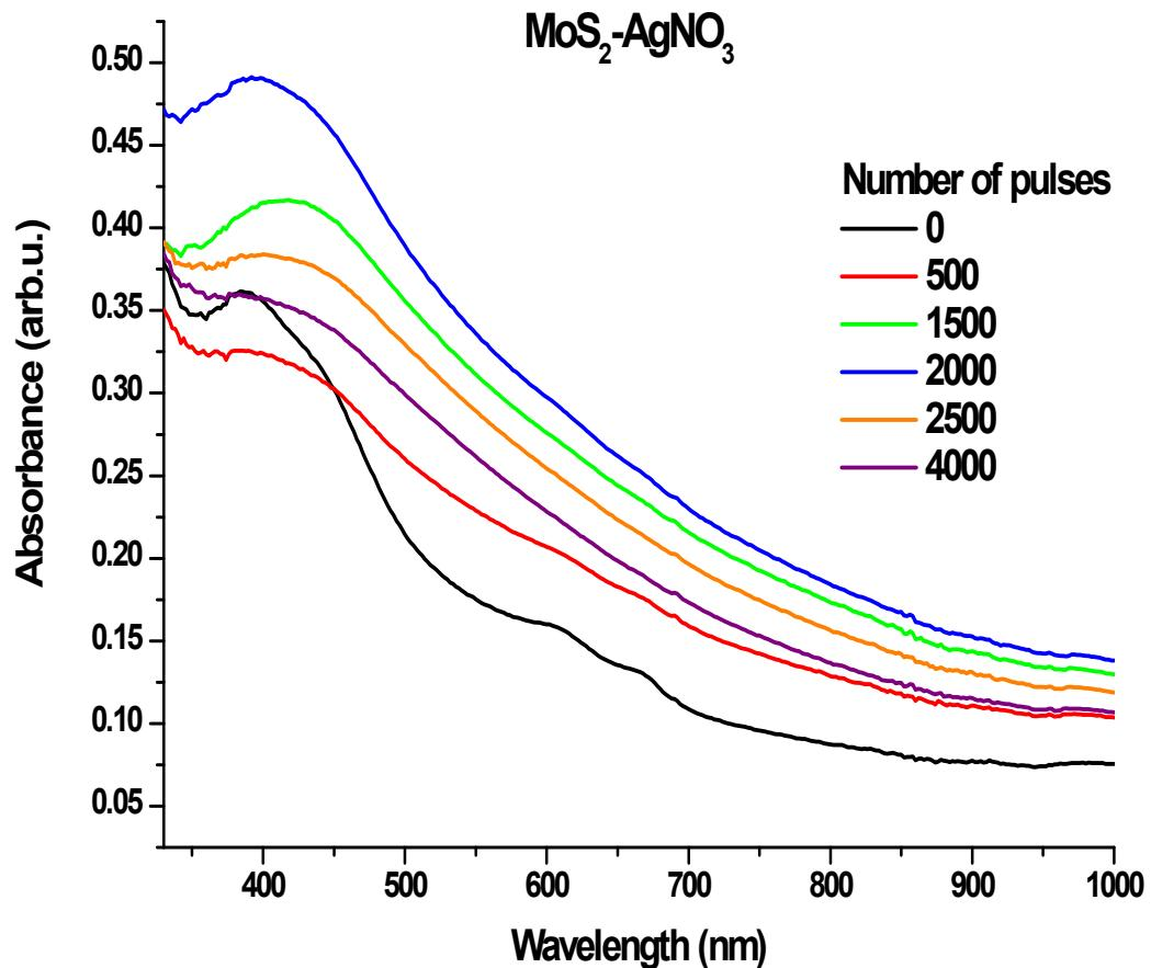
**Fig. S6:** UV-vis absorption spectra of pristine MoS<sub>2</sub>-AgNO<sub>3</sub> dispersions in water, irradiated with different numbers of 100mJcm<sup>-2</sup> UV pulses.
