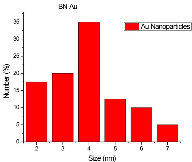
**Fig. S10:** Size distribution of BN-Au NPs, produced by a single, of 100mJcm<sup>-2</sup>, UV pulse.
