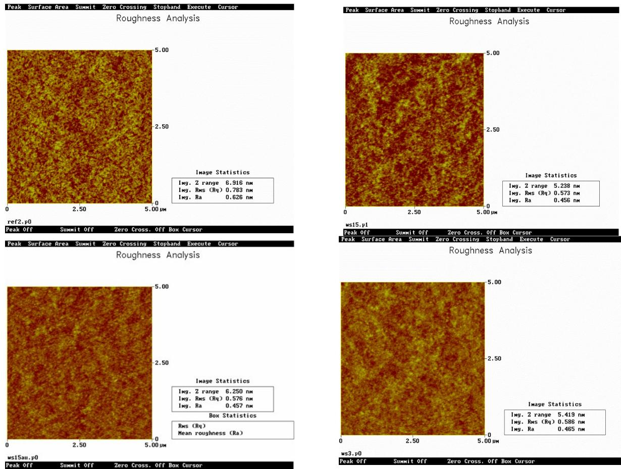
**Figure S14:** AFM images of four different devices tested a) PCDTBT:PC<sub>71</sub>BM, b) PCDTBT:1.5% (v/v) WS<sub>2</sub>:PC<sub>71</sub>BM, c) PCDTBT:1.5% (v/v) WS<sub>2</sub>-Au NPs:PC<sub>71</sub>BM and d) PCDTBT:2.5% (v/v) WS<sub>2</sub>:PC<sub>71</sub>BM. The rms roughness is 0.783 nm, 0.573 nm, 0.576 nm and 0.586 nm respectively.
