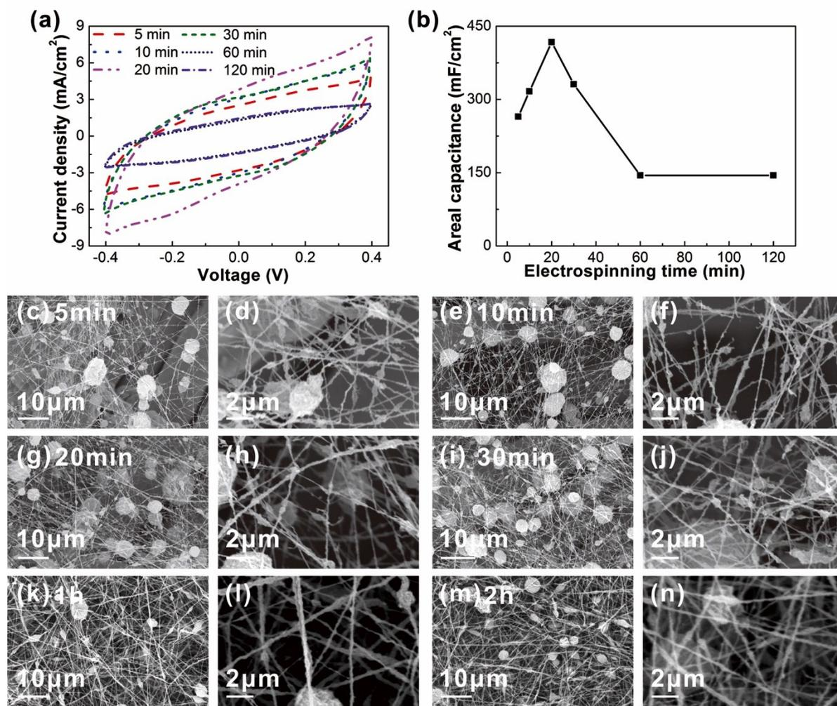
**Fig. S2** CV (a) curves and the summary real capacitance (b) of the C-Web@Ni-Cotton supercapacitor fabrics obtained by using different lengths of electrospinning time and tested in 1M Na<sub>2</sub>SO<sub>4</sub> liquid electrolyte. The scan rate is 10 mV/s. SEM images of the carbon nanoweb obtained by using different lengths of electrospinning time from 5 min (c) (d), 10 min (e) (f), 20 min (g) (h), 30 min (i) (j), 1 h (k) (l) to 2 h (m) (n).
