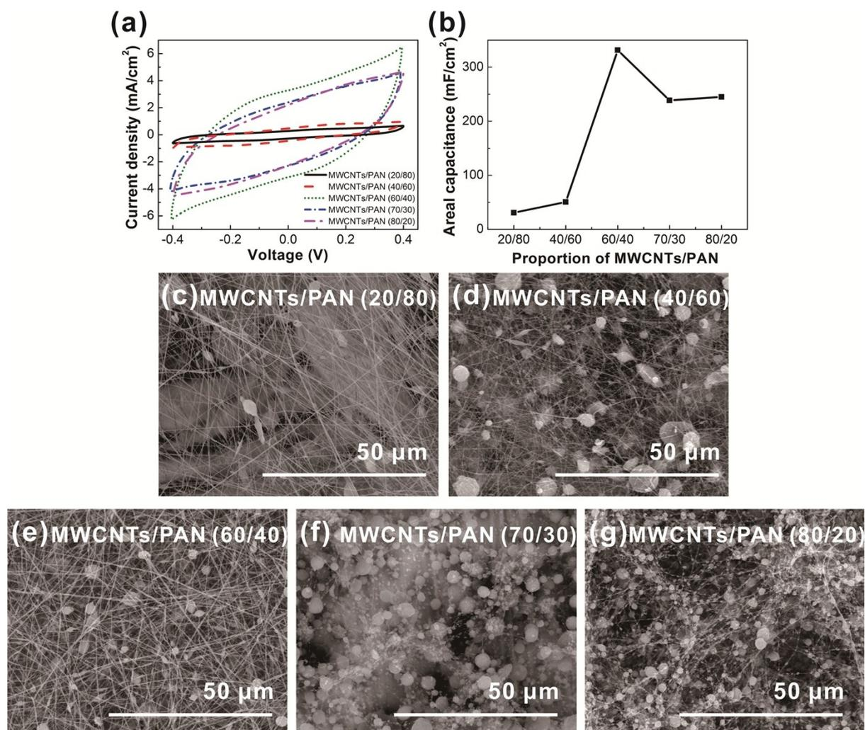
**Fig. S3** CV curves (a) and the summary of areal capacitance (b) of C-Web@Ni-Cotton supercapacitor fabrics obtained by using different MWCNTs/PAN proportions of electrospinning solutions and tested in 1M Na<sub>2</sub>SO<sub>4</sub> liquid electrolyte. The scan rate is 10 mV/s. SEM images (c)-(g) of the carbon nanofiber webs by using different MWNTs/PAN proportions.
