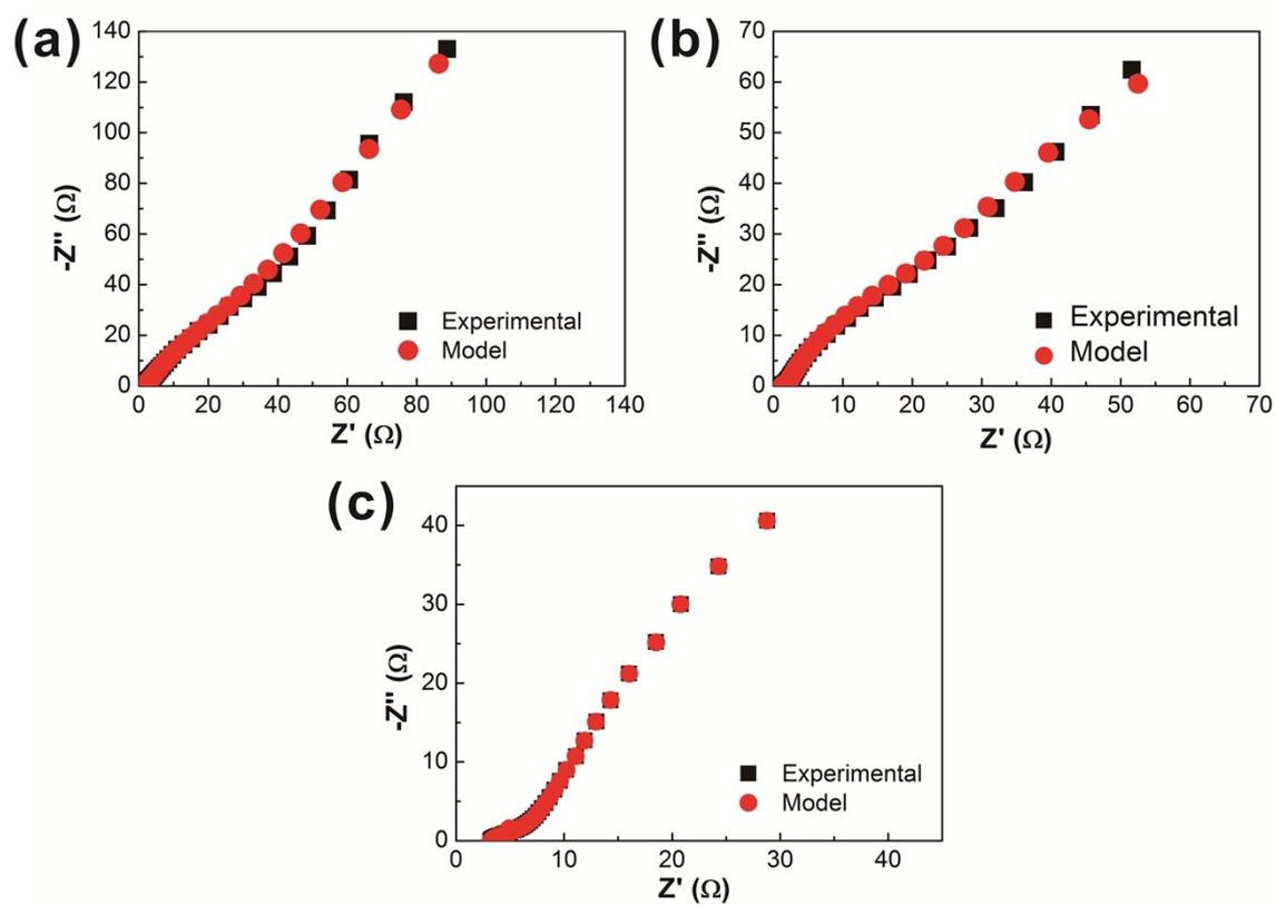
**Fig. S4** Experimental (black curve) and modeled EIS plots for the samples (a) before and (b) after 3000 cycles tested in liquid electrolyte and the (c) solid-stated supercapacitor fabric.
