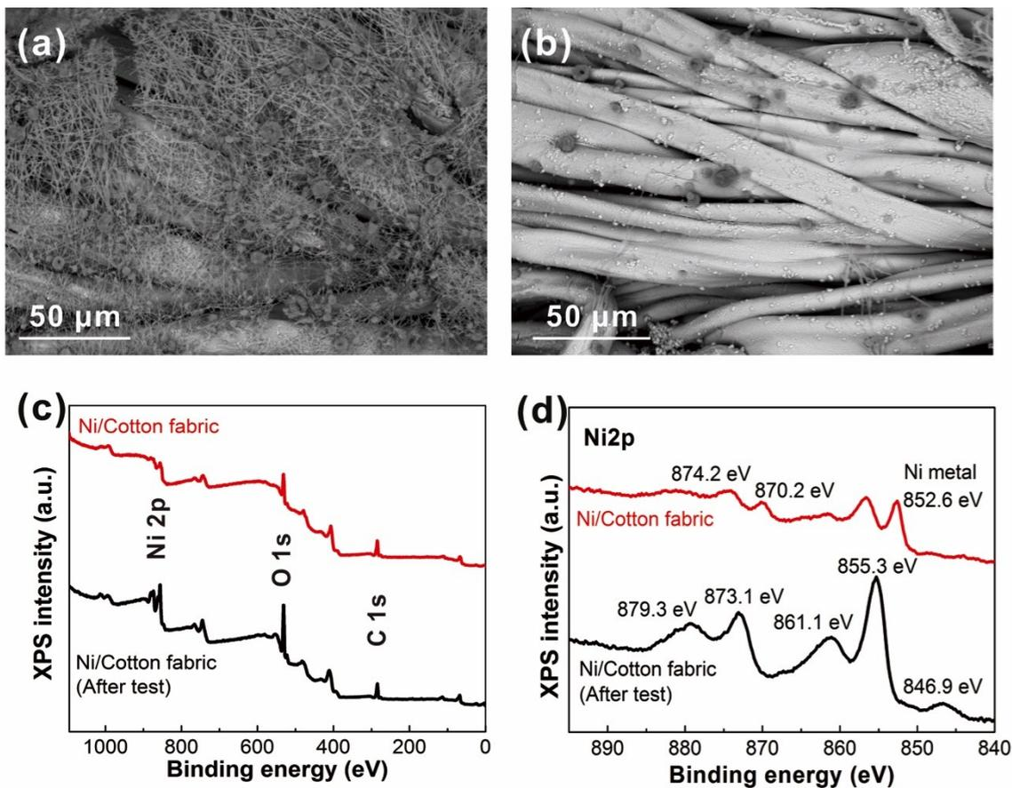
**Fig. S5** SEM images of the C-Web@Ni-Cotton fabric electrode (a) and the Ni-Cotton current collector (b) after electrochemical retention test. XPS spectra across a wide scan (c) and Ni2p XPS spectra (d) of the Ni-Cotton fabric before (red line) and after (black line) electrochemical test.
