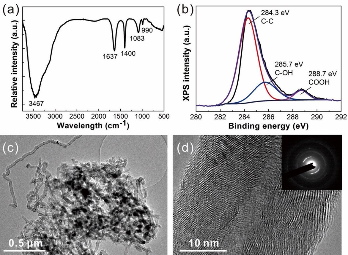
**Fig. S1** (a) IR spectra and (b) C1s core level XPS spectrum of the treated MWCNTs. (c) TEM image and (d) HRTEM image of the treated MWCNTs. The insert graph in (d) is the electron diffraction pattern.
