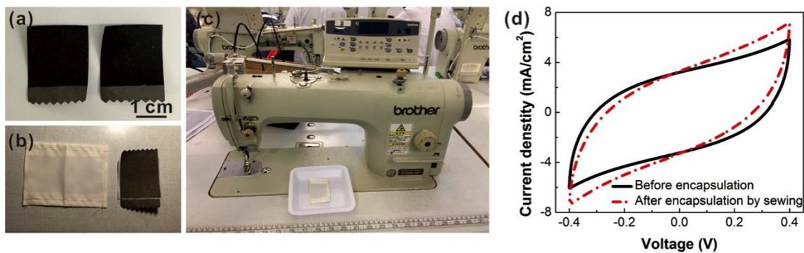
**Fig. S6** Photographs of C-Web@Ni-Cotton fabric electrodes with large dimension (a), components for assembling the supercapacitor fabrics (b) and sewing machine (brand: Brother) that used for the integration of the fabric device into commercial fabrics (c). (d) CV curves of the supercapacitor fabrics before and after encapsulation by sewing technology.
