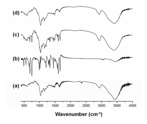
**Fig. S1.** FTIR spectra of sCD (a), chalcone (b), their physical mixture (c) and complex (d).
