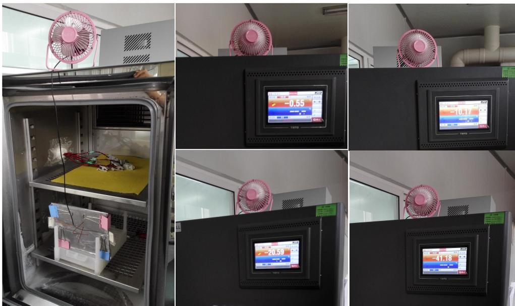
**Fig. S8** A line linkage image between hybrid batteries and electric fan (left); An electric fan is powered by two hybrid  $\text{Mg}^{2+}/\text{Li}^{+}$  pouch devices at varied low temperature of 0 (middle up), -10 (right up), -20 (middle down), and -40 °C (right down).
