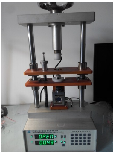
Figure S6. The photograph of the semiconductor powder resistivity apparatus. The pressure used here was 5 MPa.
