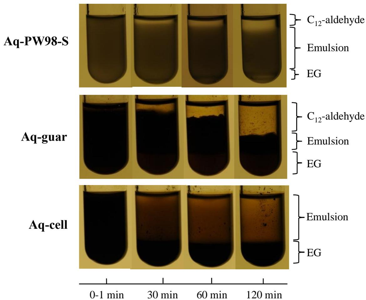
Fig. S11. Macroscopic appearance and evolution profile of  $C_{12}$ -aldehyde/EG emulsions stabilized by Aq-PW98-S, Aq-guar and Aq-cell. Emulsification conditions as in Fig. S10.
