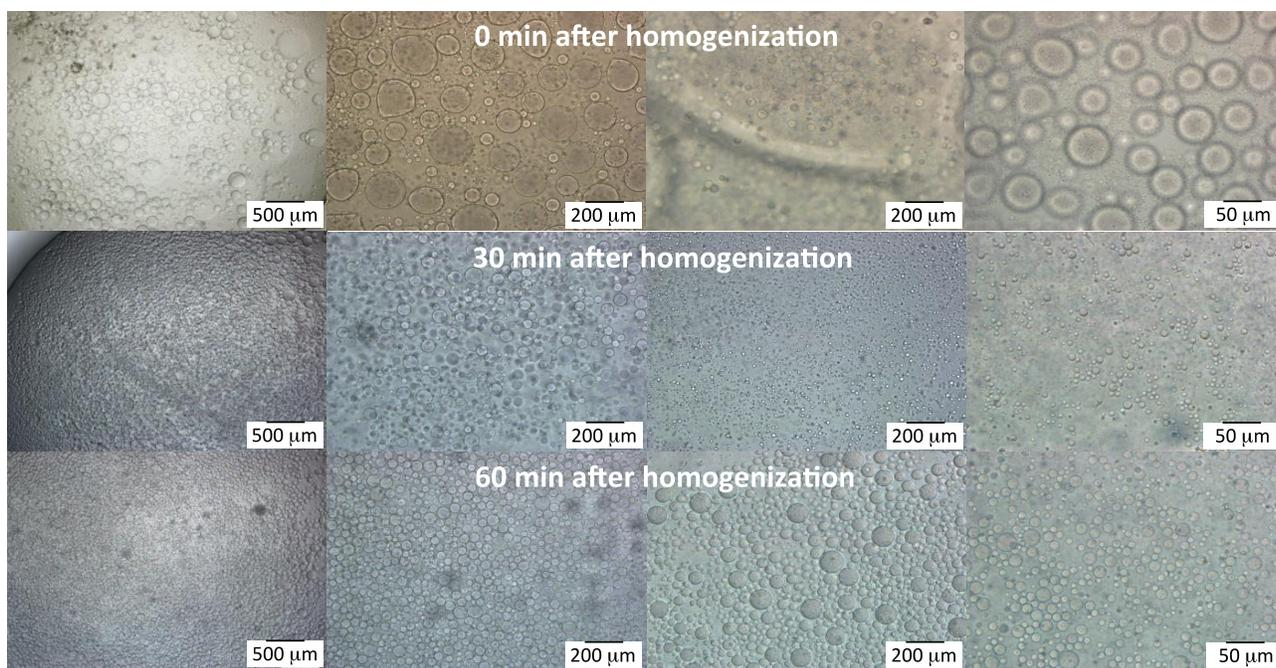
Fig. S12. Microscopic appearance and evolution profile of  $C_{12}$ -aldehyde/EG emulsions stabilized by Aq-PW98-S. Emulsification conditions as in Fig. S10.
