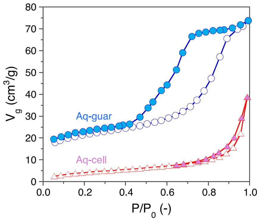
Fig. S8. N<sub>2</sub> adsorption/desorption isotherms at 77 K for Aq-guar and Aq-cell.
