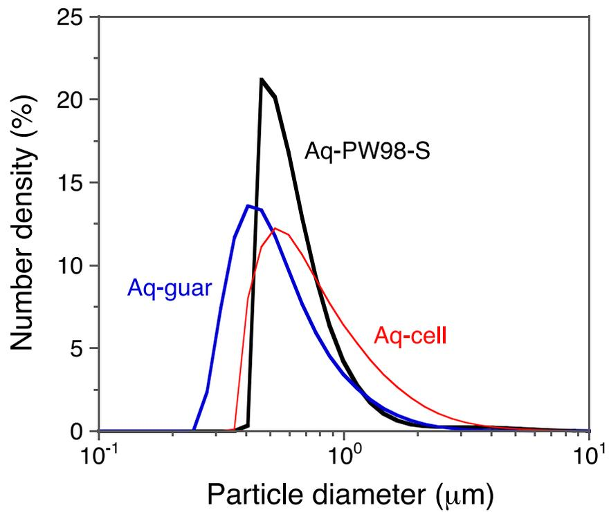
Fig. S9. Particle size distributions (PSDs) of Aq-PW98-S, Aq-guar and Aq-cell (supernatant phase).
