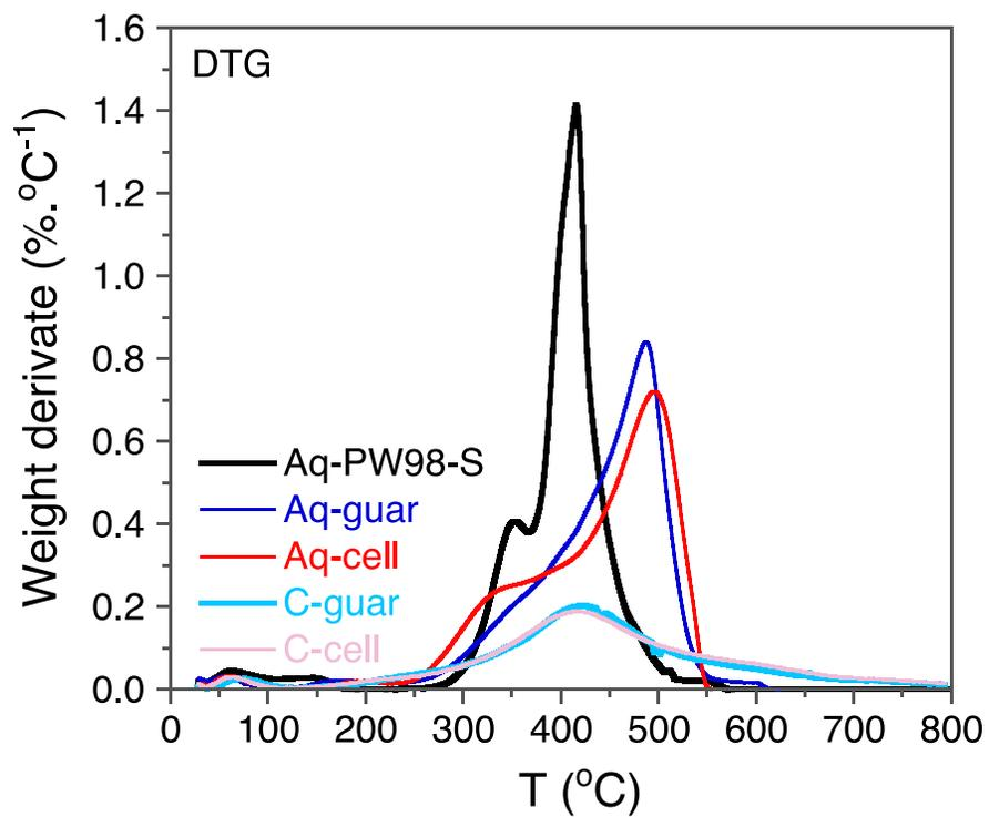
Fig. S7. TGA / DTG profiles for Aq-PW98-S, Aq-guar and Aq-cell.
