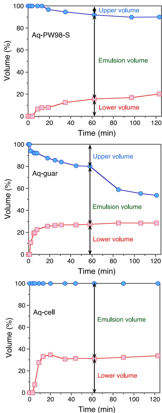
Fig. S10. Time-evolution of the emulsion volume for the  $C_{12}$ -aldehyde/EG system stabilized by Aq-PW98-S, Aq-guar and Aq-cell. Emulsification conditions: 45 °C, 10 mmol  $C_{12}$ -aldehyde, 20 mmol EG, catalyst loading providing 10  $\mu\text{molH}^+$ , homogenization at 13,000 rpm for 5 min.
