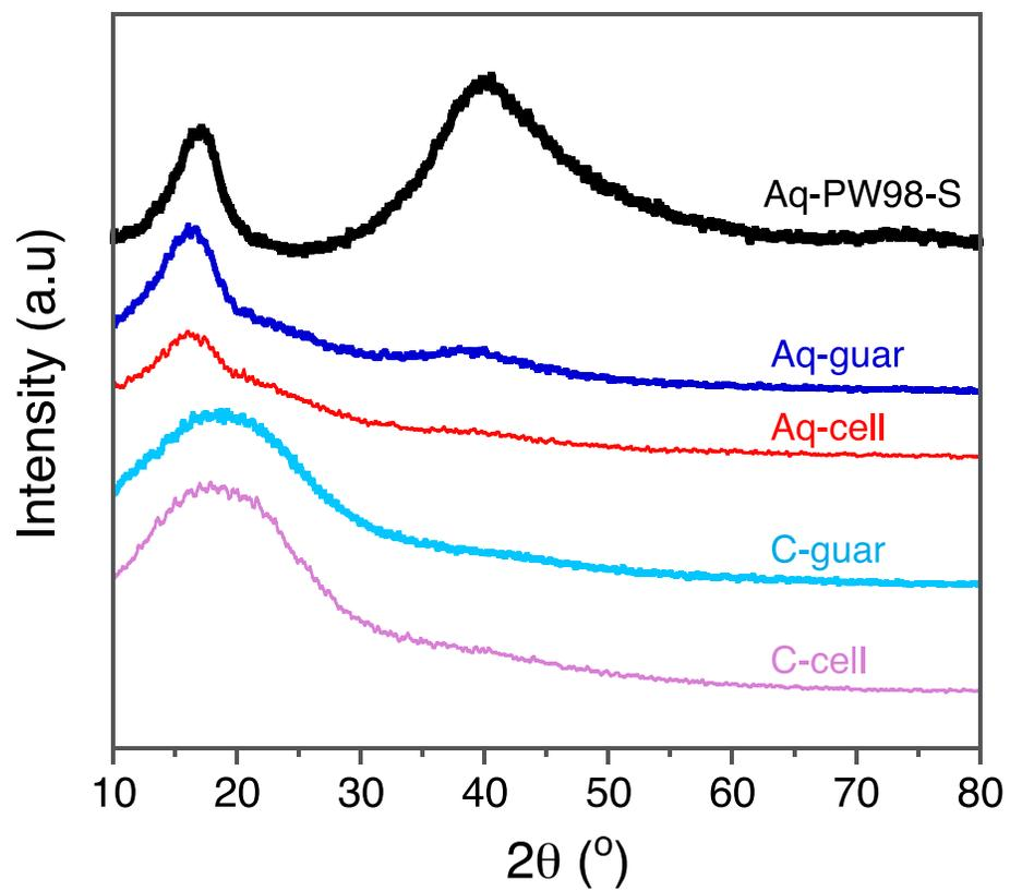
Fig. S2. XRD patterns of Aq-PW98-S, Aq-guar, Aq-cell, C-guar and C-cell.
