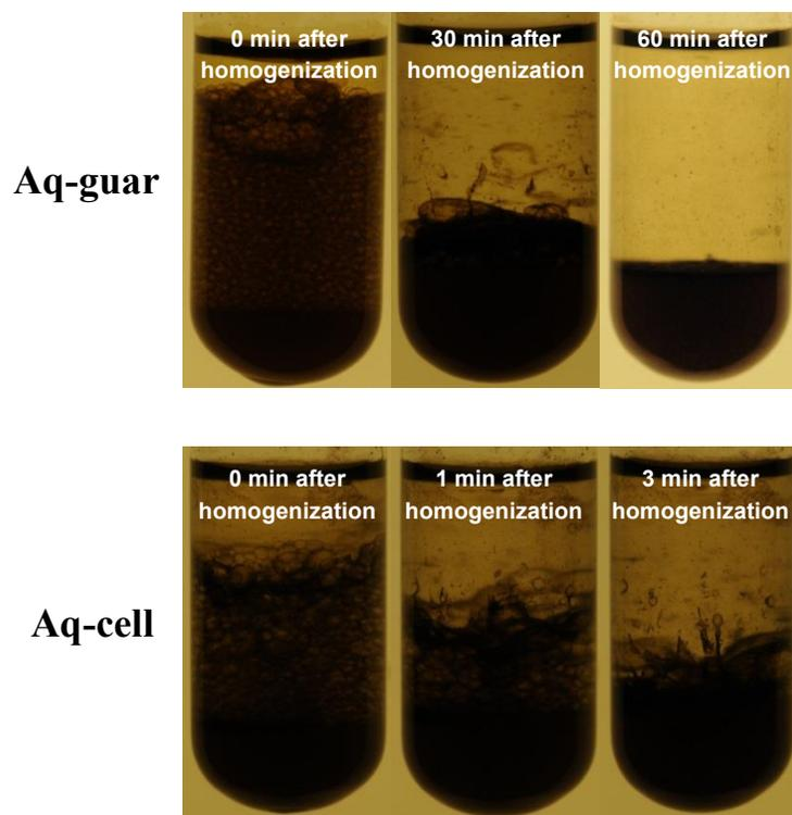
Fig. S13. Macroscopic appearance and evolution profile of  $C_{12}$ -aldehyde/EG emulsions stabilized by Aq-guar and Aq-cell at low particle weight loading. Emulsification conditions: 45 °C, 10 mmol  $C_{12}$ -aldehyde, 20 mmol EG, 0.1 wt.% catalyst loading, homogenization at 13,000 rpm for 5 min.
