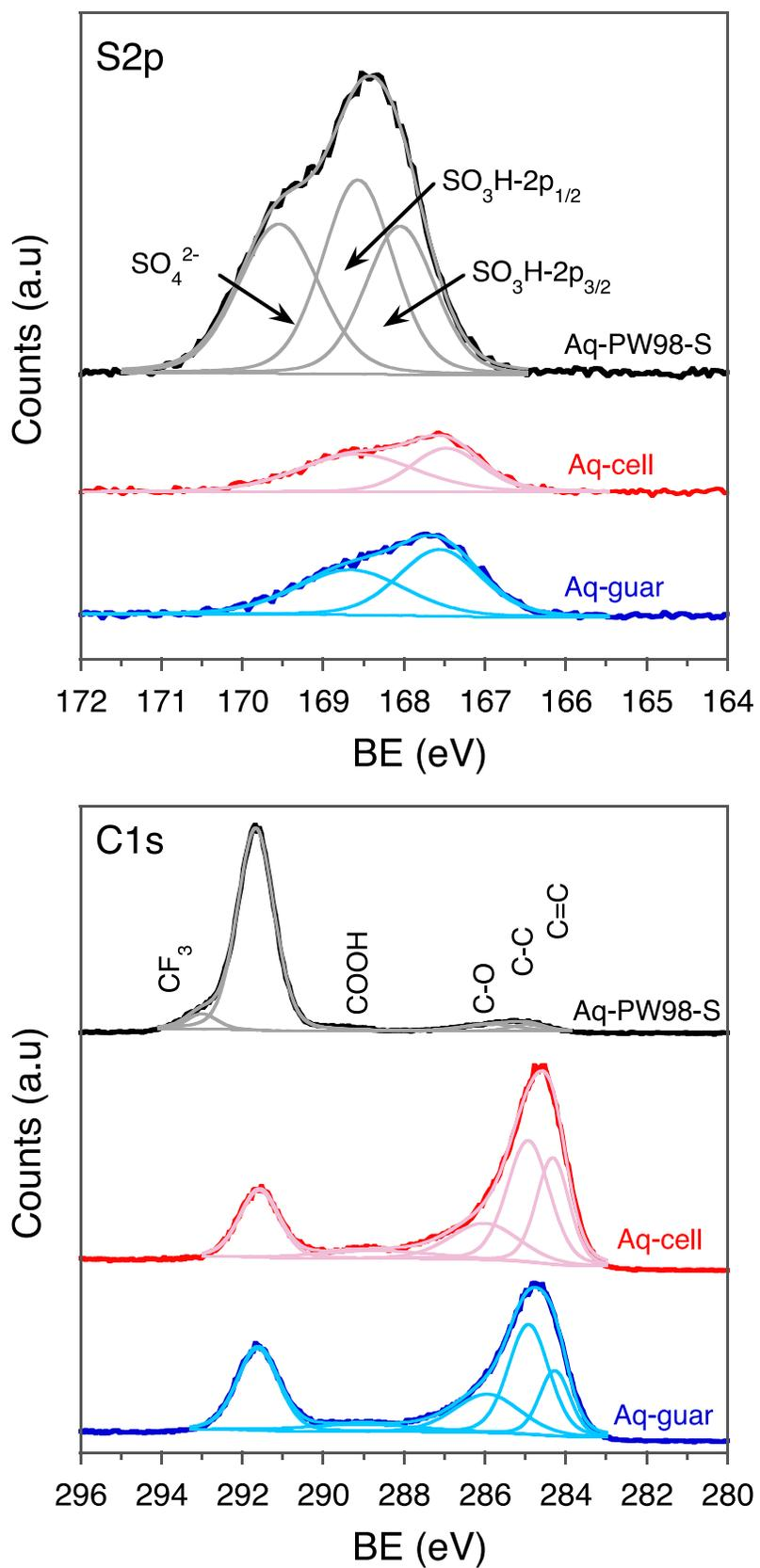
Fig. S6. S2p (top) and C1s (bottom) XPS spectra of Aq-PW98-S, Aq-guar and Aq-cell.
