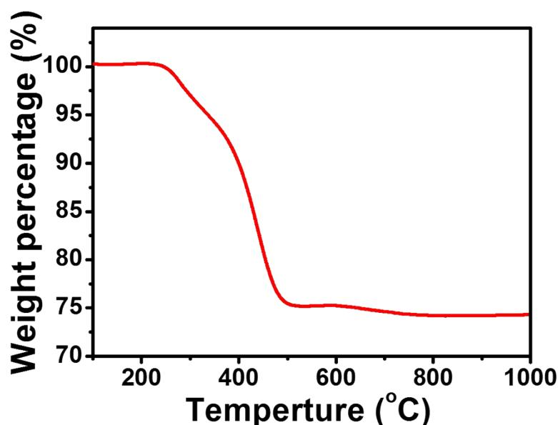
**Figure S1.** Thermogravimetric (TGA) curve of CNT/FeO<sub>x</sub> in air.
