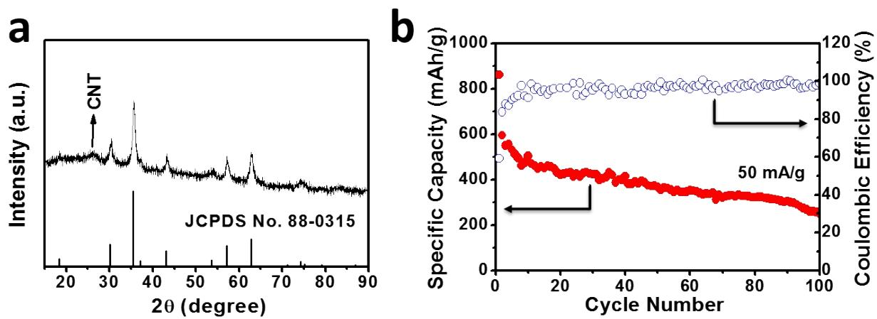
**Figure S6.** (a) XRD pattern of annealed composite suggesting the formation of  $\text{Fe}_3\text{O}_4$  phase. (b) Cycling performance and coulombic efficiency of annealed composite at a specific current of 50 mA/g. The material was prepared by annealing as-prepared CNT/ $\text{FeO}_x$  composite under Ar at 500°C for 2 h.
