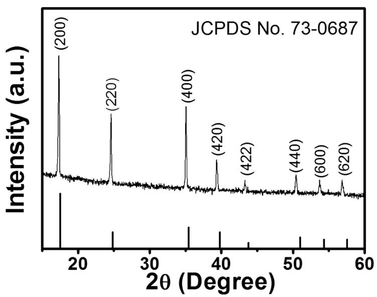
**Figure S2.** XRD pattern of  $\text{Na}_x\text{FeFe}(\text{CN})_6$  powders.
