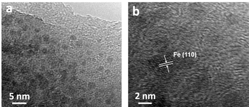
**Figure S4.** TEM images of CNT/FeO<sub>x</sub> hybrid materials after the initial discharge. These dark particles correspond to metallic Fe as the discharge product.
