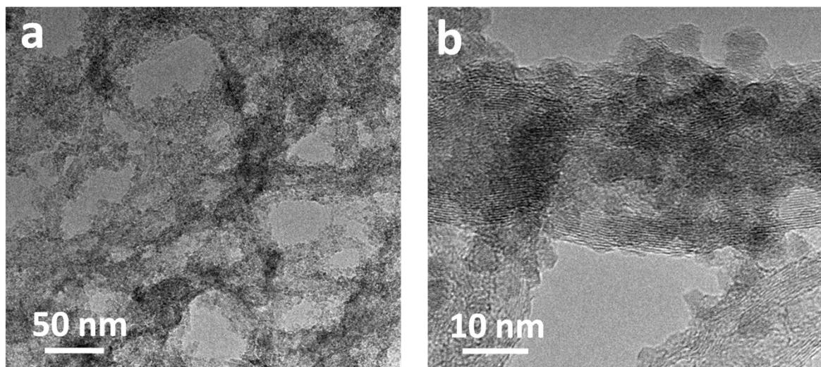
**Figure S5.** TEM images of CNT/FeO<sub>x</sub> after 100 charge/discharge cycles. They suggest the preservation of electrode material integrity even after extended cycling.
