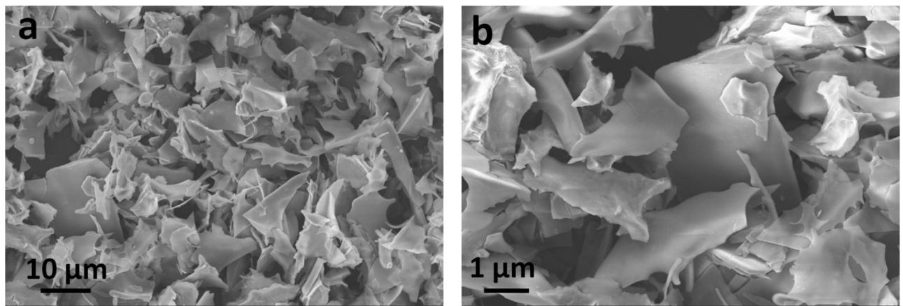
**Figure S3.** SEM images of  $\text{FeO}_x$  prepared in the absence of CNTs.
