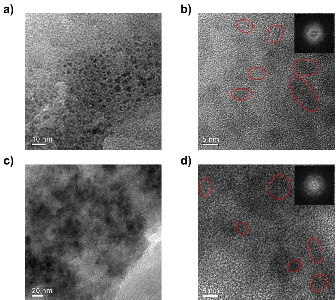
**Figure S15** TEM images of selected carbon-rich areas of **C-1a** depicted in a) and b) and of **C-1b** depicted in c) and d). The images in b) and d) magnify areas exhibiting crystalline germanium, which are marked by red circles. The insets in b) and d) show the electron diffraction patterns of the crystalline germanium.
