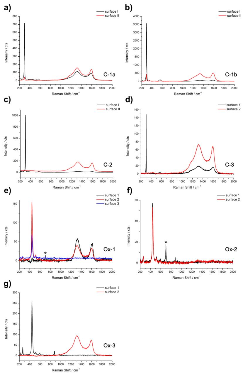
**Figure S12** Raman spectra of a) C-1a b) C-1b, c) C-2, d) C-3, e) Ox-1, f) Ox-2 and g) Ox-3 at selected surfaces of the samples. The asterisks \* in e) and f) mark Raman bands assigned to tetragonal GeO<sub>2</sub>.
