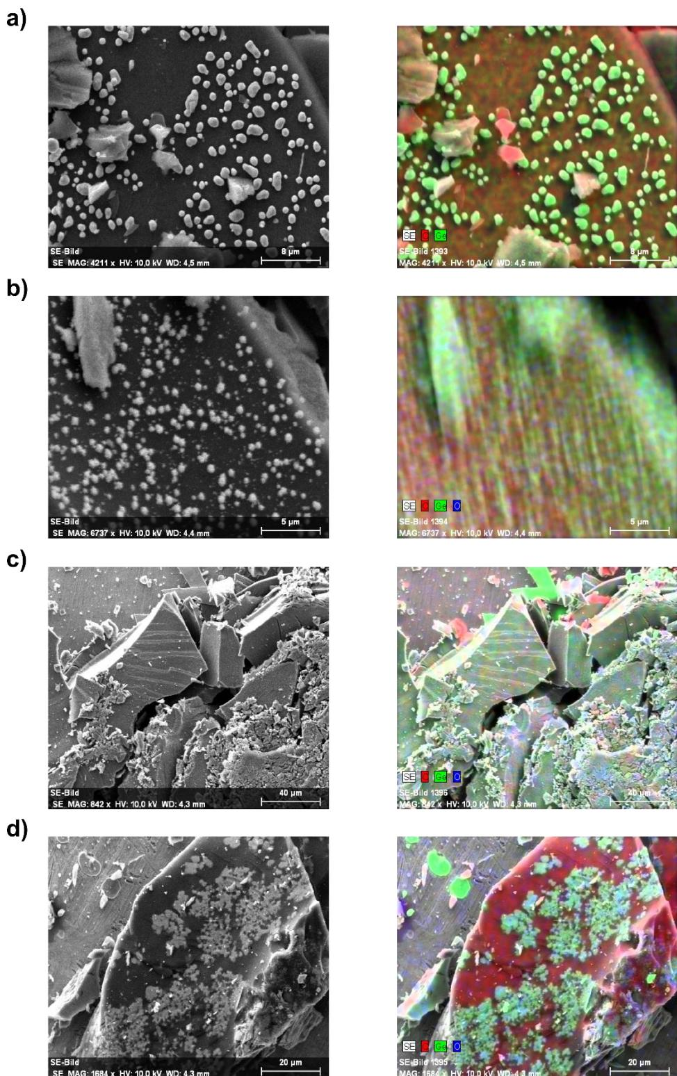
**Figure S13** SEM images (left) with EDX mapping (right) of a) C-1a, b) C-1b, c) C-2 and d) C-3. The EDX mapping colors green, red and blue denote germanium, carbon and oxygen, respectively.
