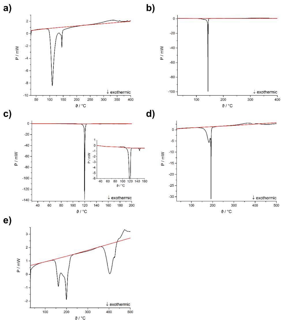
**Figure S11** Differential scanning calorimetry (black curve) measurement of a) amorphous material of **1**, b) crystals of **(1)<sub>3</sub>**, c) crystals of **2** (**1**)<sub>4</sub> · *n*-pentane, d) amorphous material of **2** and e) amorphous material of **3**. Baseline (red curve) was added in order to distinguish exothermic and endothermic processes.
