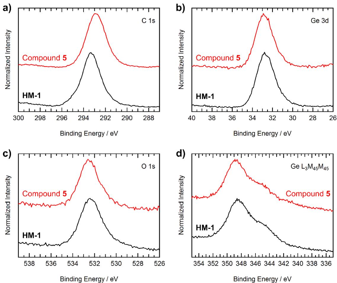
**Figure S7** XPS core-level spectra of **HM-1** and compound **5**, showing emission from the a) C 1s, b) Ge 3d, and c) O 1s levels as well as d) Auger spectra arising from the Ge L<sub>3</sub>M<sub>45</sub>M<sub>45</sub> transition. Spectra are normalized to the same height and offset for clarity. In addition, the binding energy in b)-d) has been corrected for the shift caused by charging.
