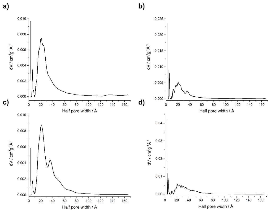
**Figure S10** Pore size distributions of: a) **C-1a**, b) **C-1b**, c) **C-2** and d) **C-3**. The pore size distributions were estimated according to the QSDFT model for slit and cylindrical pores using the adsorption branch for carbon materials.
