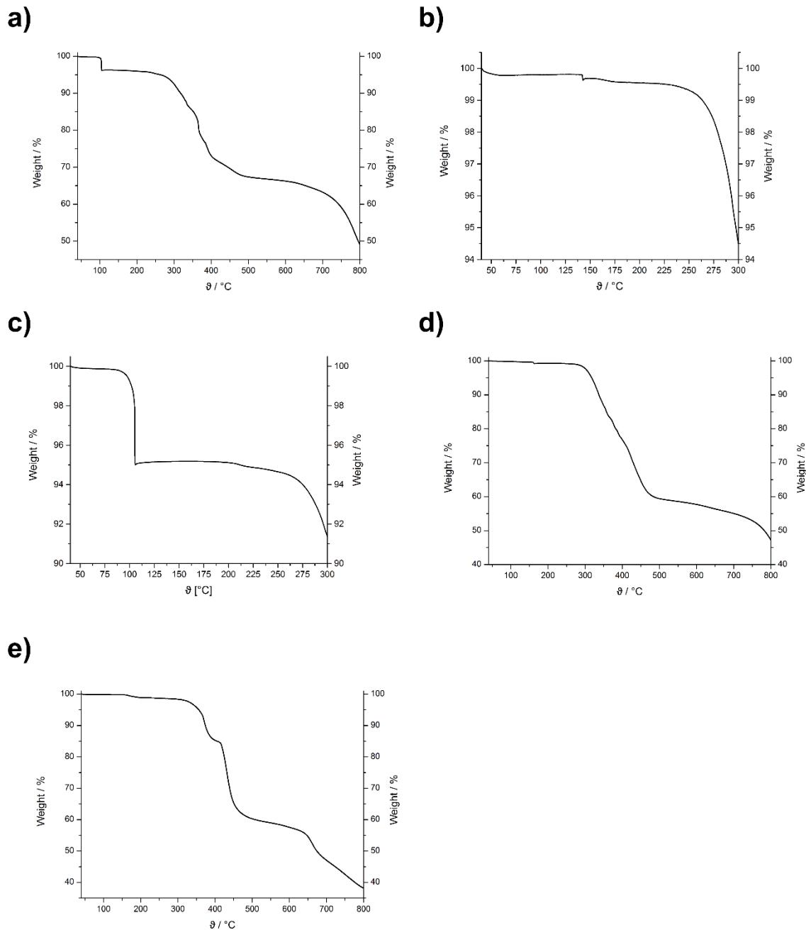
**Figure S3** Thermal gravimetric analysis of a) amorphous material of **1**, b) crystals of **(1)<sub>3</sub>**, c) crystals of **2·(1)<sub>4</sub> · n-pentane**, d) amorphous material of **2** and e) amorphous material of **3**. The first weight loss step in a) with an onset temperature of 104  $^{\circ}\text{C}$  is assigned to the release of residual solvents within the amorphous material of **1** as similarly detected for crystals of **2·(1)<sub>4</sub> · n-pentane** in c).
