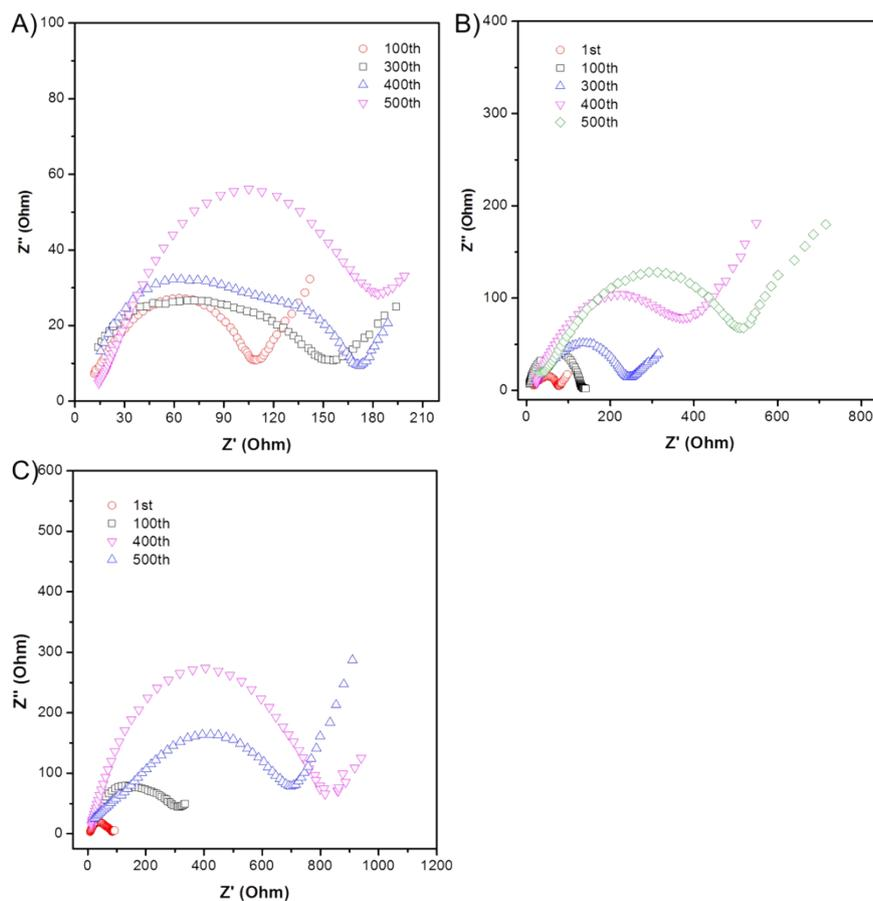
**Figure S7.** Nyquist plots of CuO electrodes at different cycle performance: (A) hierarchical CuO mesocrystals; (B) CuO nanosheets, and (C) CuO nanorods.
