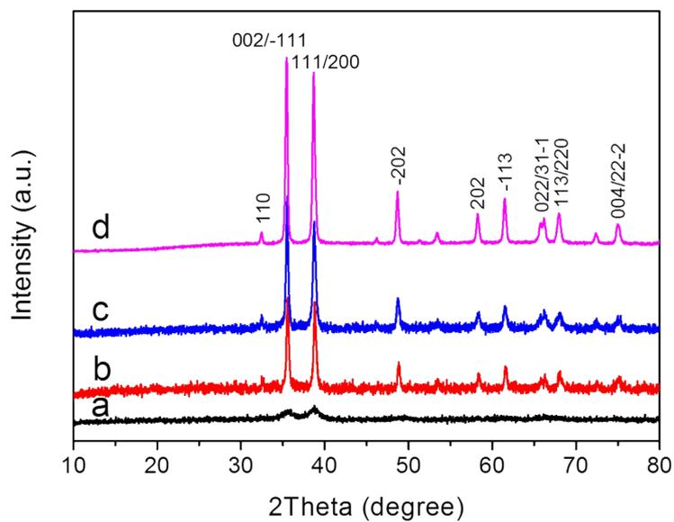
**Figure S3.** XRD patterns of as-prepared CuO samples at different reaction times: (a) 0.5 h; (b) 2 h; (c) 4 h; (d) 12 h. The diffraction peaks in b-d can be perfectly indexed to the monoclinic CuO (JCPDS Card 48-1548).
