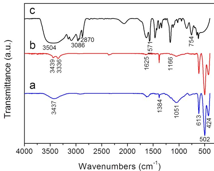
**Figure S2.** FT-IR spectra of (a) CuO, (b) [Bmim]Cl/CuO, and (c) [Bmim]Cl.
