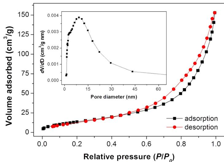
**Figure S6.** Nitrogen adsorption/desorption isotherms and the corresponding pore size distribution for the 3D hierarchical CuO mesocrystals. The BET surface area is about 45.2 m<sup>2</sup>/g.
