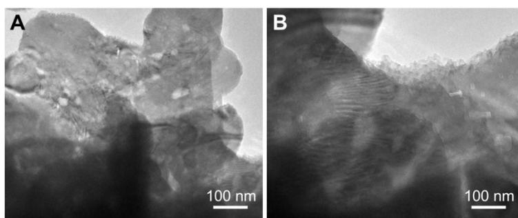
**Figure S8.** TEM images of the CuO mesocrystalline electrodes after 500 cycles.
