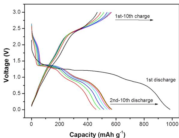
**Figure S5.** Galvanostatic charge-discharge curves of hierarchical CuO mesocrystalline electrode for the first ten cycles between 0.01 and 3 V at a current density of  $67 \text{ mA g}^{-1}$ .
