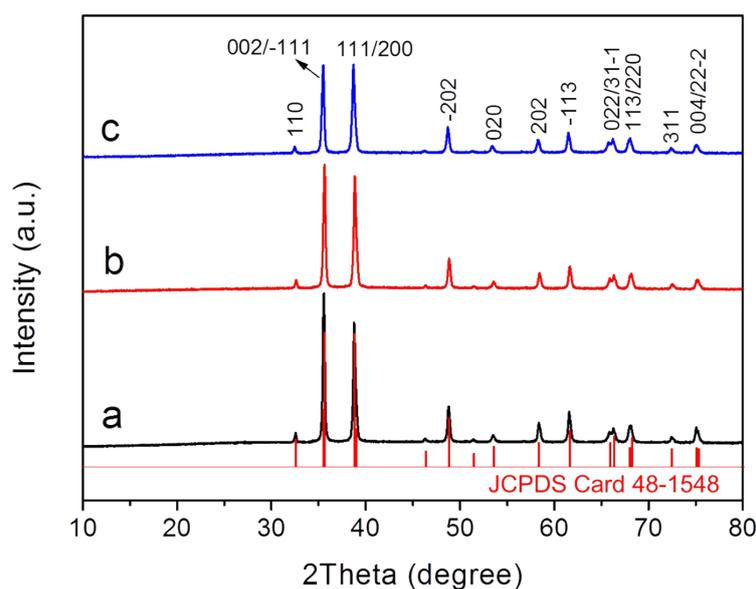
**Figure S1.** XRD patterns of as-prepared CuO samples at different concentrations of [Bmim]Cl: (a) 0 mmol, butterfly-like nanosheets; (b) 1 mmol, hierarchical mesocrystals composed of nanosheets; (c) 5 mmol, nanorods. All the diffraction peaks can be perfectly indexed to the monoclinic CuO (JCPDS Card 48-1548).
