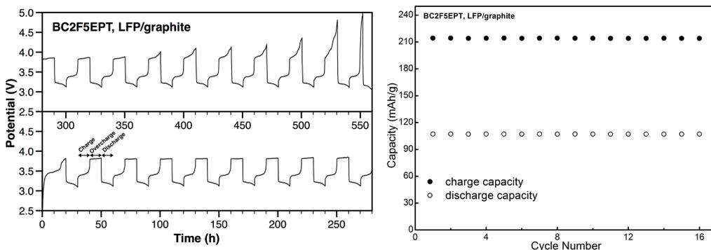
**Figure S6.** Potential vs. time (left) and capacity vs. cycle number (right) for 100% overcharge cycling of BC2FEPT in LFP/graphite coin cells. BC2FEPT was incorporated into 1.2 M  $\text{LiPF}_6$  in EC/EMC (3:7 wt. ratio) at 0.08 M; 100% overcharge cycling was performed at a rate of C/10.
