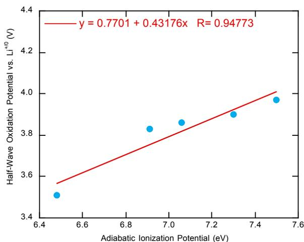
**Figure S4.** A plot of half-wave oxidation potentials for the first oxidation event for redox shuttle candidates EPT, BCF3EPT, BC2F5EPT, DCNEPT, and DNO2EPT in 1.2 M LiPF<sub>6</sub> in EC/EMC (3:7 wt. ratio) recorded at a scan rate of 100 mV/sec vs. the adiabatic IPs calculated at the B3LYP/6-311G(d,p) level of theory.
