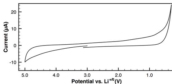
**Figure S3.** Cyclic voltammogram of 1.2 M LiPF<sub>6</sub> in EC/EMC (3:7 wt. ratio) recorded at a scan rate of 100 mV/sec.
