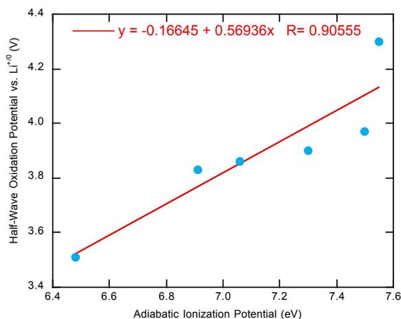
**Figure S5.** A plot of half-wave oxidation potentials for the first oxidation event for redox shuttle candidates EPT, BCF3EPT, BC2F5EPT, DCNEPT, DNO2EPT, and OFEPT in 1.2 M LiPF<sub>6</sub> in EC/EMC (3:7 wt. ratio) recorded at a scan rate of 100 mV/sec vs. the adiabatic IPs calculated at the B3LYP/6-311G(d,p) level of theory.
