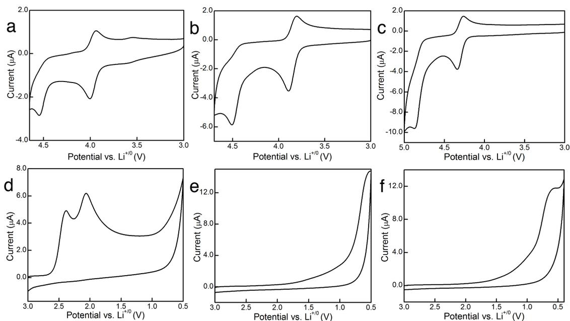
**Figure S2.** Cyclic voltammograms of DNO<sub>2</sub>EPT (a,d), BC<sub>2</sub>F<sub>5</sub>EPT (b,e), and OFEPT (c,f) at 0.3 mM in 1.2 M LiPF<sub>6</sub> in EC/EMC (3:7 wt. ratio) recorded at a scan rate of 100 mV/sec showing irreversible second oxidations in some cases (a, b, and c) and irreversible reductions in others (d, e, and f).
