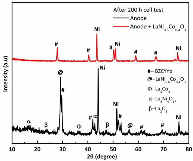
**Fig. 5.** The XRD analysis of the anode faces of single cells after cell test revealed that the Ni catalyst remained active with high crystallinity. Further, no degradation of the constituent phases of the anodes with and without catalyst layer was observed.
