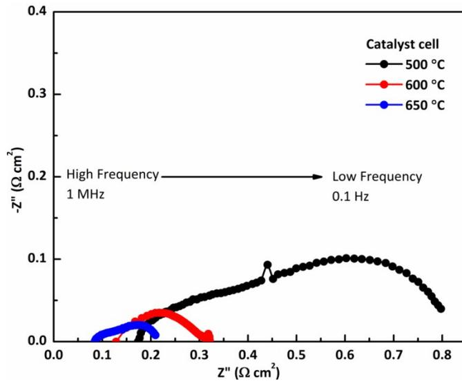
**Fig. 3.** The Impedance spectra of anode supported single cell with catalyst layer ( $\text{LaNi}_{0.6}\text{Co}_{0.4}\text{O}_3/\text{NiO-BZCYYb/BZCYYb/LSCF-BZCY}$ ) under open circuit conditions: The ohmic and polarization resistances were calculated to be 0.08, 0.13, 0.18  $\Omega \text{ cm}^2$  and 0.14, 0.21, 0.62  $\Omega \text{ cm}^2$  at 650, 600, and 500  $^\circ\text{C}$ , respectively.
