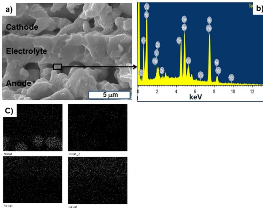
**Fig. 4.** (a) SEM cross-sectional image of a single cell without additional catalyst layer operated under methane fuel for 200 h. (b) A small area EDX is shown and all the initial constituent elements were present at the interface with almost no carbon deposition. (c) The area EDX map of Fig. 4a is shown. It was observed that all the elements remained at their respective positions with no any migration.
