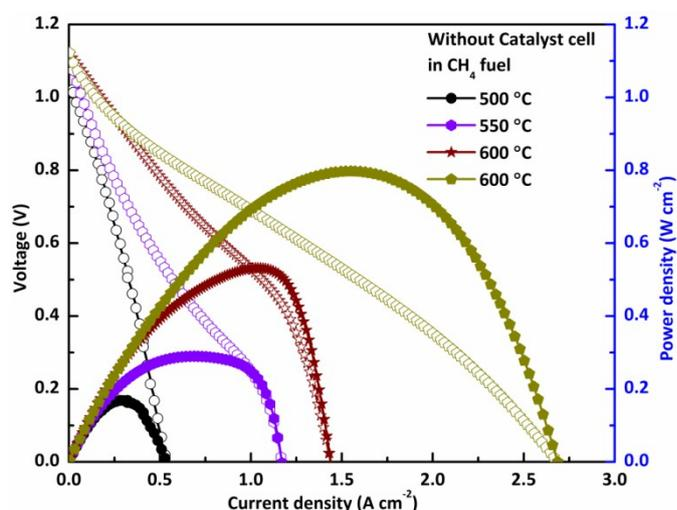
**Fig. 1.** *I*-*V* and *I*-*P* curves of anode supported single cell without a catalyst layer (NiO-BZCYYb/BZCYYb/LSCF-BZCY) under a humidified CH<sub>4</sub> fuel: The maximum power densities were 0.797, 0.53, 0.29, and 0.16 W cm<sup>-2</sup> at 650, 600, 550, and 500 °C, respectively.
