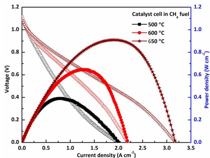
**Fig. 2.** *I*-*V* and *I*-*P* curves of anode supported single cell with a catalyst layer ( $\text{LaNi}_{0.6}\text{Co}_{0.4}\text{O}_3/\text{NiO-BZCYYb/BZCYYb/LSCF-BZCY}$ ) under a humidified CH<sub>4</sub> fuel: The maximum power densities were 0.92, 0.66, and 0.39 W cm<sup>-2</sup> at 650, 600, and 500 °C.
