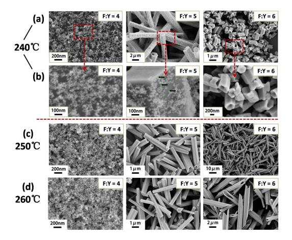
*Figure S4* SEM images of the samples at different proportions of F/Y and temperature conditions (a-d).Hydrothermal time was 12 h, only PST was added.
