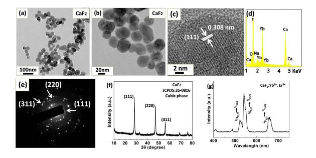
*Figure S6* CaF<sub>2</sub>:Yb<sup>3+</sup>, Er<sup>3+</sup>upconversion nanoparticles (30-40 nm) of TEM (a), local magnification (b), HRTEM (c), EDS (d) and SAED (e). X-ray diffraction pattern (f) and photoluminescence (g) is corresponding to cubic phase of CaF<sub>2</sub>.
