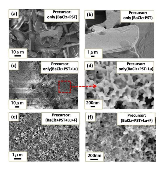
*Figure S9* SEM images for BaLuF<sub>5</sub>:Yb<sup>3+</sup>, Er<sup>3+</sup> precursors (a-f).
