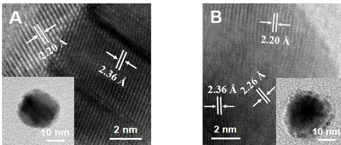
Fig. S5 HR-TEM images of a single Au@Ag (A) and a single Au@Pt@Ag (B) on GO nanosheets.
