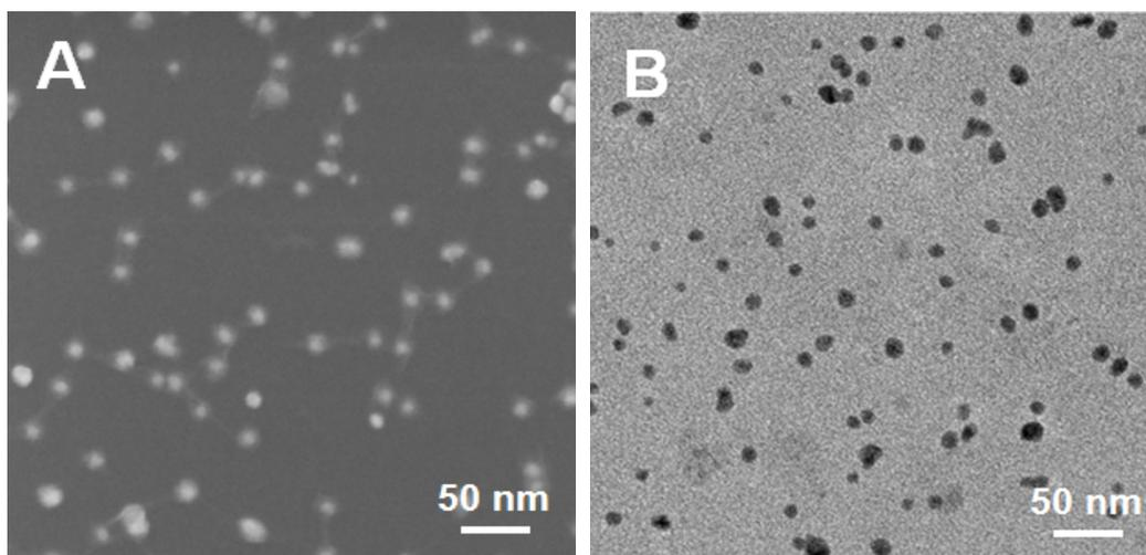
**Fig. S1** SEM (A) and TEM (B) images of GO/Au nanocomposites.
