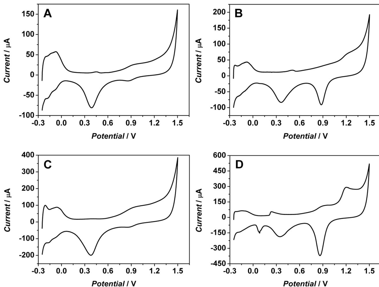
Fig. S6 Cyclic voltammograms of (A) Au@Pt, (B) Au@Pt@Au, (C) GO/Au@Pt and (D) GO/Au@Pt@Au catalysts in nitrogen-saturated 0.5 M  $\text{H}_2\text{SO}_4$ . Scan rate: 50  $\text{mV s}^{-1}$ .
