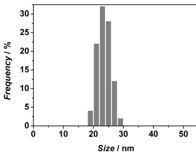
**Fig. S4** Size-histogram of Au@Pt@Au nanoparticles on GO nanosheets based on TEM measurement.
