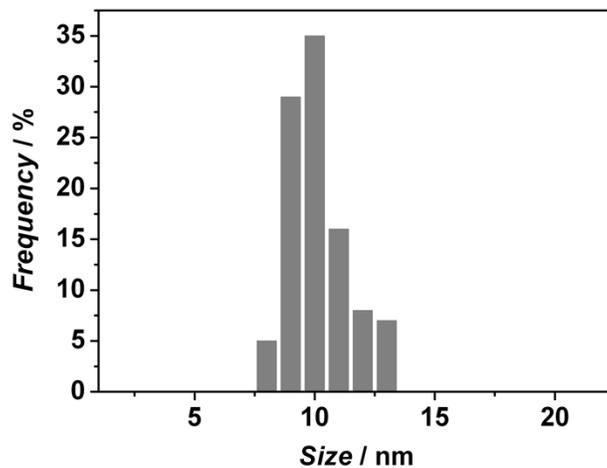
**Fig. S2** Size-histogram of Au nanoparticles on GO nanosheets based on TEM measurement.
