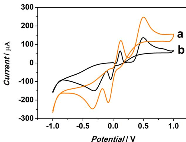
**Fig. S8** Cyclic voltammograms of (a) GO/Au@Pt@Au-modified GCE with two exposed metal surfaces (Au and Pt) consisting of the Au core, Pt inner shell, and Au protuberances outer shell and (b) GO/Au@Pt@Au(s)-modified GCE with one exposed metal surface (Au) consisting of the Au core, Pt inner layer and smooth Au outer shell on GO nanosheets in nitrogen-saturated PBS (0.1 M pH 7.4) + 5 mM H<sub>2</sub>O<sub>2</sub>. Scan rate: 50 mV s<sup>-1</sup>.
