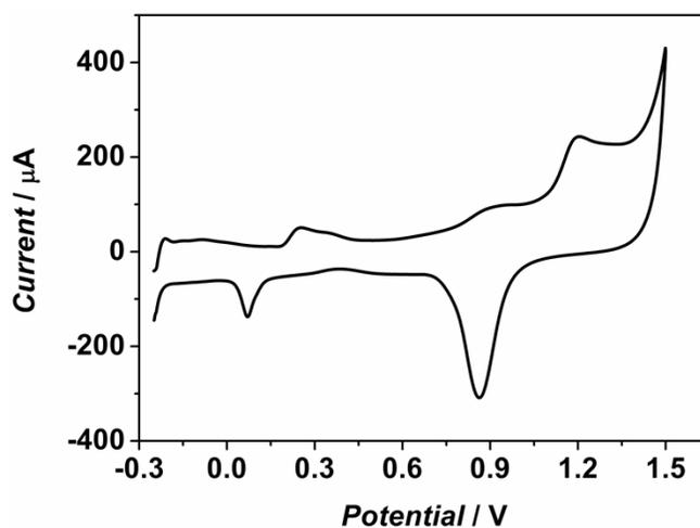
Fig. S7 Cyclic voltammograms of GO/Au@Pt@Au(s) catalysts with one exposed metal surface (Au) consisting of the
