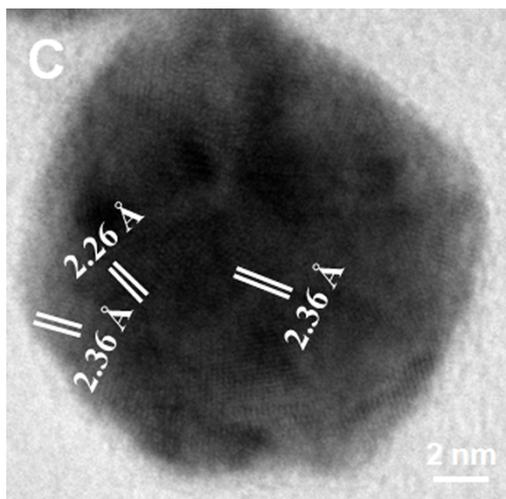
**Fig. S3** (A-B) TEM images of GO/Au@Pt@Au(s) nanocomposites without sodium citrate in the last reaction step; (C) HR-TEM images of a single Au@Pt@Au(s) nanoparticle with a Au core, Pt inner layer and smooth Au outer shell on GO nanosheets.
