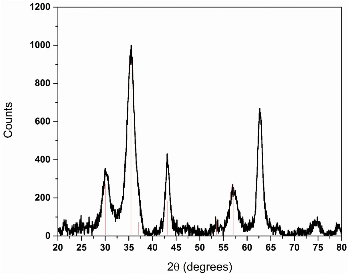
Figure 1: XRD-measurement of Fe<sub>3</sub>O<sub>4</sub>-oleate capped nanoparticles (black line) and the standard cubic phase with relative intensities according to JPDS 16-629 (red).
