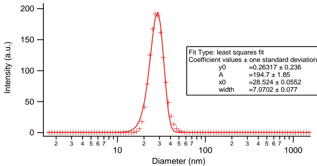
**Figure 4: Hydrodynamic diameter of IO-ReL<sub>2</sub>. The red crosses are the datapoints obtained by DLS measurement and the gaussfitting is visualized by a red line. The parameters acquired from the fitting are given in the textbox.**
