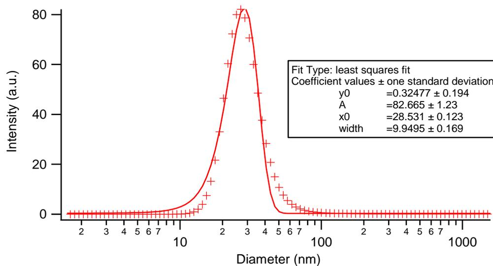
**Figure 3: Hydrodynamic diameter of IO-ReL<sub>1</sub>. The red crosses are the datapoints obtained by DLS measurement and the gaussfitting is visualized by a red line. The parameters acquired from the fitting are given in the textbox.**
