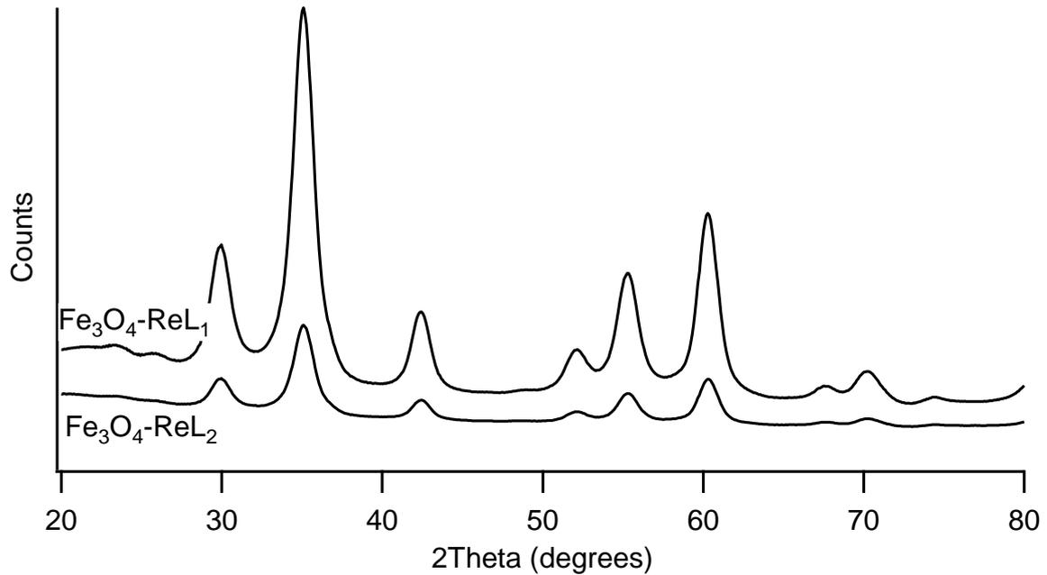
**Figure 2: powder X-ray diffraction of  $\text{Fe}_3\text{O}_4\text{-ReL}_1$  and  $\text{Fe}_3\text{O}_4\text{-ReL}_2$ . The pattern follows nicely the crystalline structure of magnetite nanoparticles (black line) and the standard cubic phase with relative intensities according to JPDS 16-629 (red).**
