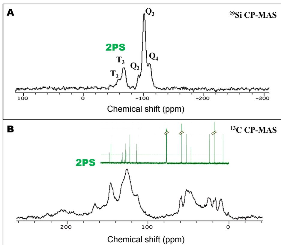
Figure S3. Solid state NMR CPMAS spectra of  $^{29}\text{Si}$  (A) and  $^{13}\text{C}$  (B) for M2PS-35 NPs.
