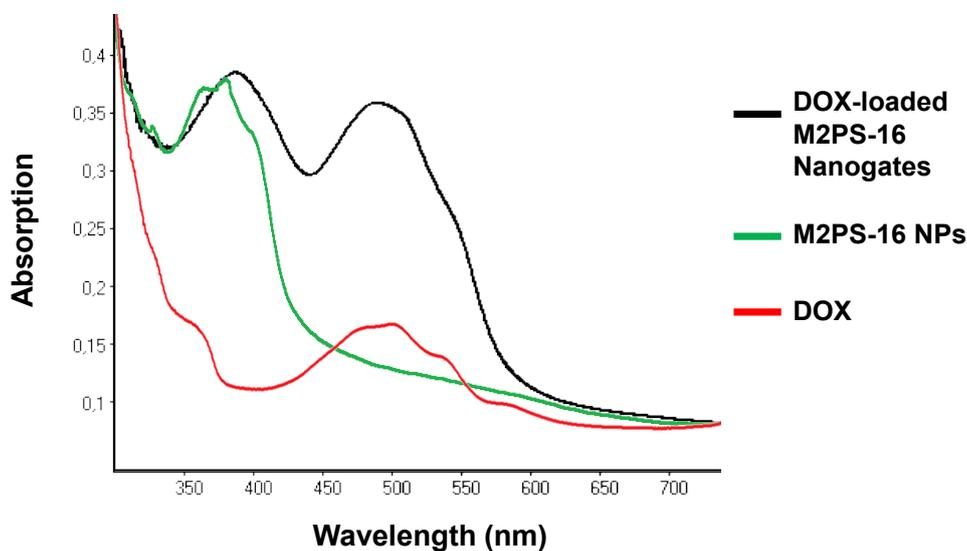
**Figure S7.** Absorption spectra comparison of DOX, M2PS-16, and DOX loaded M2PS-16 nanogates in water, depicting the DOX encapsulation in the M2PS mesopores.
