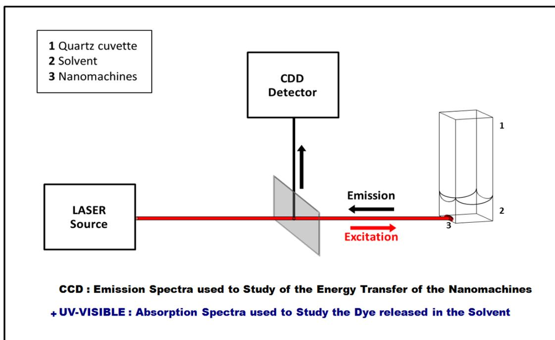
**Scheme S1.** Representation of the two-photon irradiation settings for the cargo release in solution. The quartz cuvette was taken out of this setting for UV-Visible measurements during the experiment.
