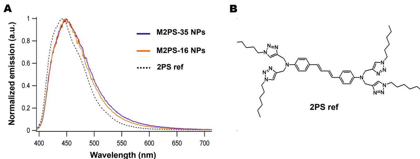
**Figure S5.** Normalized fluorescence emission spectra of M2PS-16 and M2PS-35 NPs (A), compared with a reference of the 2PS precursor in ethanol (B). The redshift of the peak of the 2PS in the NPs indicates the aggregation of the chromophore.
