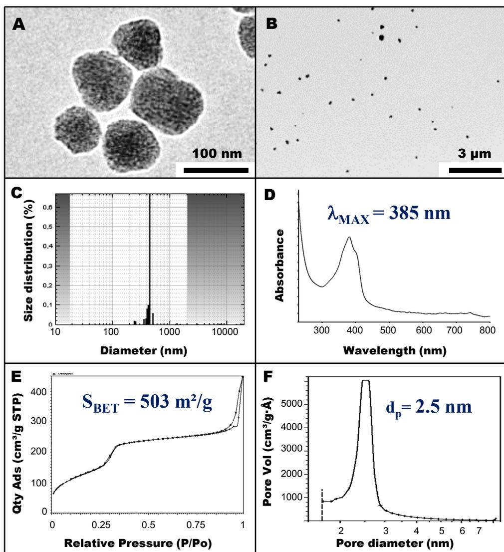
**Figure S1.** M2PS-35 nanogates characterization via TEM (A-B), DLS (C), UV-Visible spectroscopy (D), and  $N_2$ -adsorption-desorption isotherm (E) BJH pore size distribution (F).
