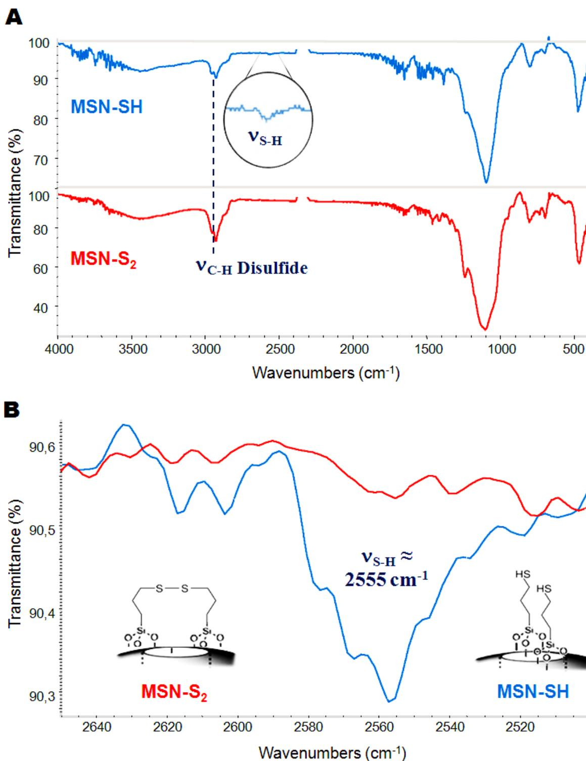
**Figure S8.** IR spectra comparison of MSN-SH and MSN-S<sub>2</sub> (after iodine addition) controls confirming the disulfide redox mechanism.
