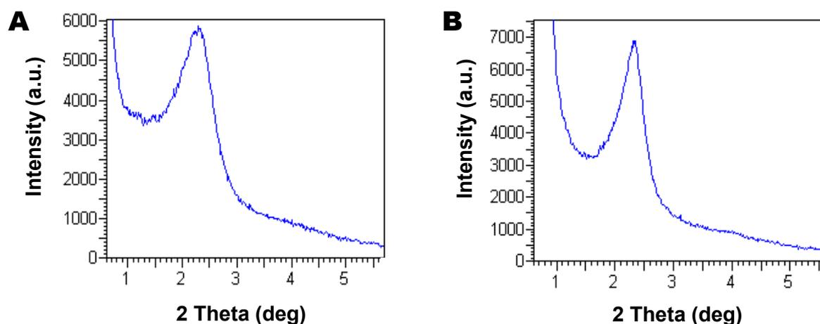
**Figure S4.** Small angle XRD patterns of M2PS-35 (A), and M2PS-16 NPs (B).
