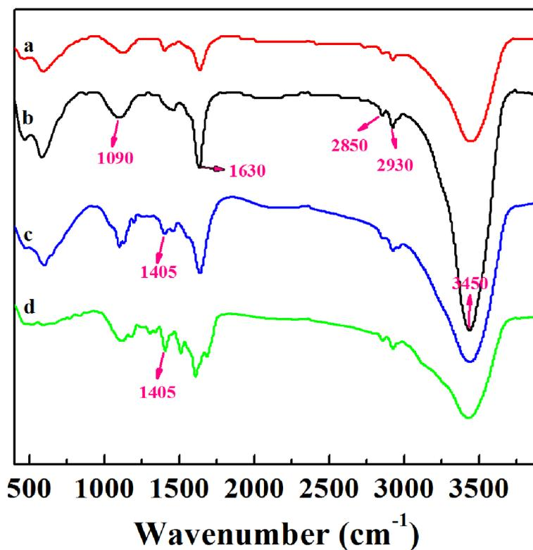
**Fig. S2** FTIR spectra of the naked Fe<sub>3</sub>O<sub>4</sub> NPs (a), Fe<sub>3</sub>O<sub>4</sub>@PEI NPs (b), Fe<sub>3</sub>O<sub>4</sub>@PEI-PEG-FA NPs (c), and FA (d).
