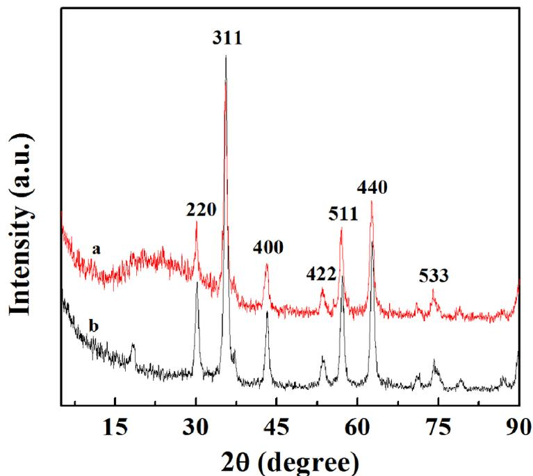
**Fig. S1** XRD pattern of the formed Fe<sub>3</sub>O<sub>4</sub>@PEI NPs (a) and naked Fe<sub>3</sub>O<sub>4</sub> NPs (b).
