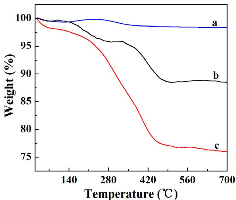
**Fig. S3** TGA curves of naked  $\text{Fe}_3\text{O}_4$  (a),  $\text{Fe}_3\text{O}_4@PEI$  (b), and  $\text{Fe}_3\text{O}_4@PEI-PEG-FA$  (c) NPs.
