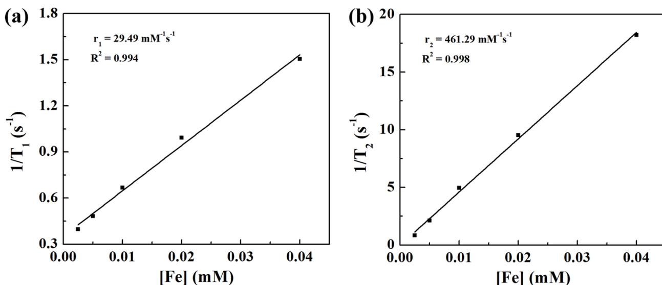
**Fig. S5** Linear fitting of  $1/T_1$  (a) and  $1/T_2$  (b) of the  $\text{Fe}_3\text{O}_4@PEI$  NPs as a function of Fe concentration.
