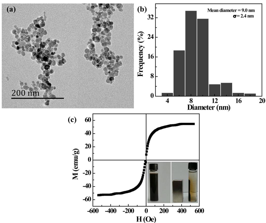
**Fig. S4** TEM image (a) and size distribution histogram (b) of the  $\text{Fe}_3\text{O}_4@PEI$  NPs and room temperature magnetization curve of  $\text{Fe}_3\text{O}_4@PEI$  NPs (c). Inset of (c) is the digital picture of the aqueous suspension of  $\text{Fe}_3\text{O}_4@PEI$  NPs before and after exposed to a magnetic field.
