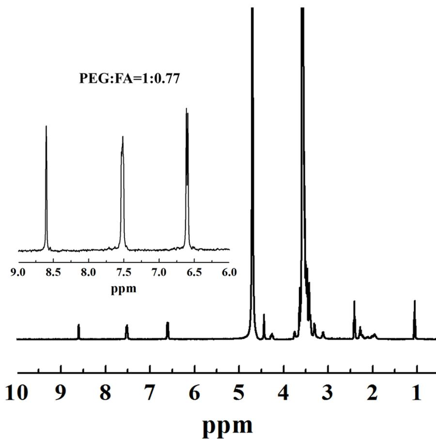
**Fig. S6**  $^1\text{H}$  NMR spectrum of PEGylated FA dissolved in  $\text{D}_2\text{O}$ .
