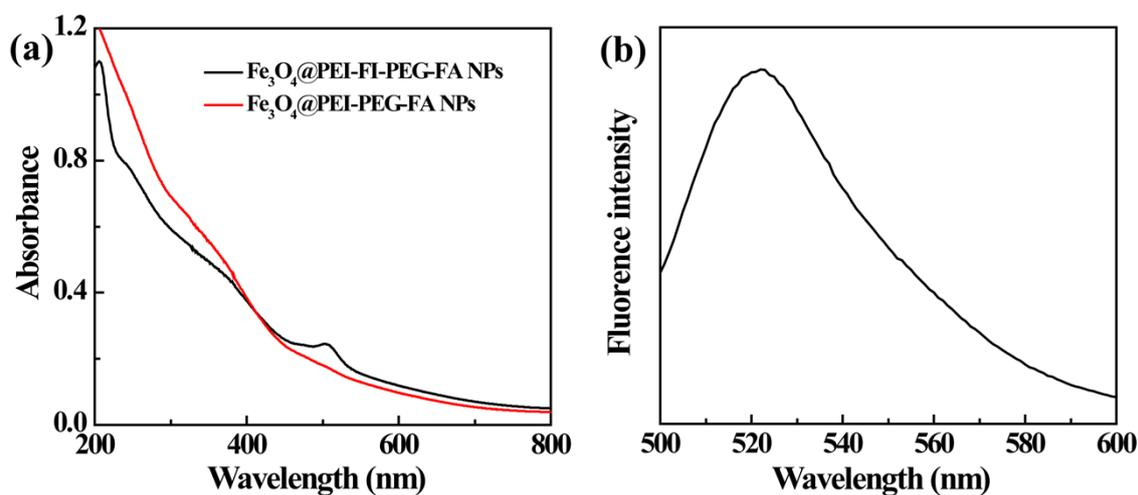
**Fig. S7** (a) UV-vis spectra of the  $\text{Fe}_3\text{O}_4@PEI-PEG-FA$  NPs and  $\text{Fe}_3\text{O}_4@PEI-FI-PEG-FA$  NPs dispersed in water; (b) fluorescent emission spectrum of the  $\text{Fe}_3\text{O}_4@PEI-FI-PEG-FA$  NPs dispersed in water.
