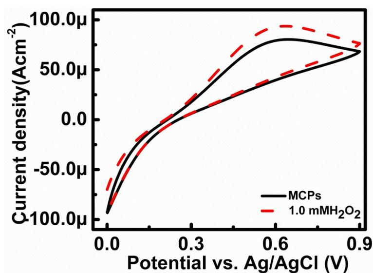
Figure S2 Cyclic voltammogram of MCPs/ITO electrode before (black) and after (red) addition of 1.0 mM  $H_2O_2$ .
