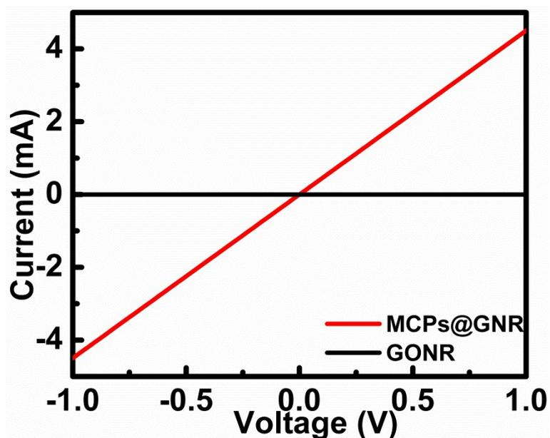
Figure S1 I-V Curves of graphene oxide nanoribbon (GONR) and graphene nanoribbon metal coordination polymer nanocomposite (MCPs@GNR) taken on pressed pallet using two probe keithley 2400 source meter.
