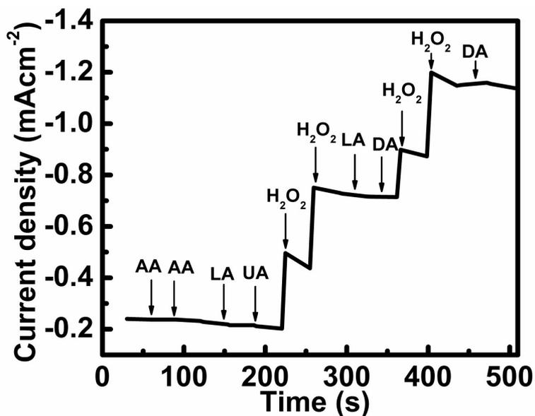
Figure S4 Amperometric response of MCPs@GNR/ITO sensor upon addition of 0.05 mM AA, LA, UA, DA and  $\text{H}_2\text{O}_2$  at 0.3 V.
