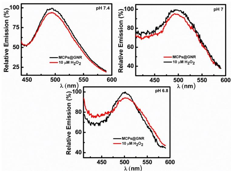
Figure S3 Fluorescence intensities of MCPs@GNR in the absence and presence of  $\text{H}_2\text{O}_2$  ( $10 \mu\text{M}$ ) at pH 7.4, 7.0 and 6.8. The results show the sensor provided the optimal sensitivity at pH 7.4 (PBS 0.1M)
