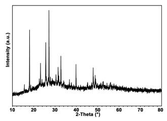
Fig. S2 XRD patterns of Cu<sub>3</sub>(TAA)<sub>3</sub>Cl<sub>3</sub>.
