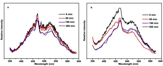
Fig. S4 PL spectra of CuS QDs, (a) amorphous, (b) crystals at different time.
