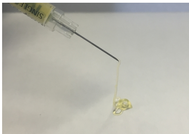
Figure S2. Injection of a 1:2 (7.8 wt%) hydrogel loaded with 100 \mu M 3W peptide through a 27G needle.
