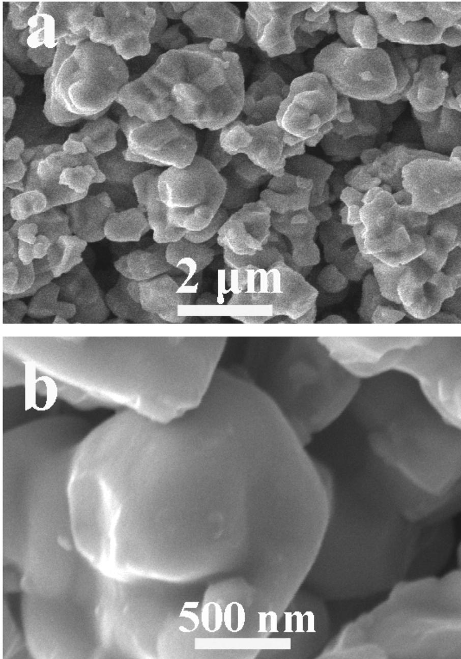
**Fig. S1** SEM images of the commercial  $\text{Mo}_2\text{C}$  particles.
