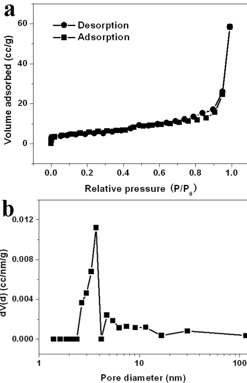
**Fig. S2** (a) N<sub>2</sub> adsorption-desorption isotherm and (b) pore size distribution of Mo<sub>2</sub>C NWs.
