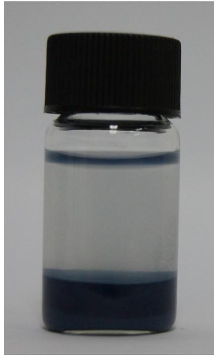
**Fig. S1** Digital photo of  $W_{18}O_{49}$  nanowire
