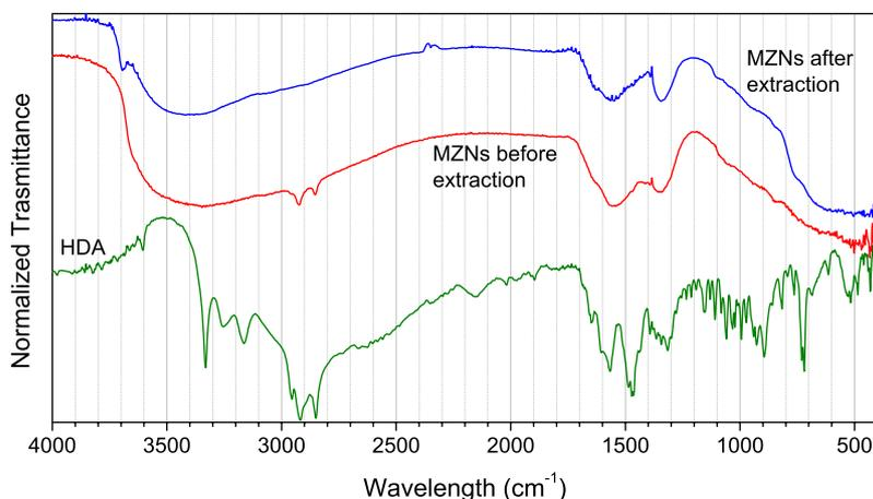
**Figure S2** IR spectra of MZNs before and after purification process. HDA spectrum is also reported.
