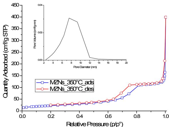
**Figure S3** Nitrogen adsorption-desorption curves of MZNs sample Z1 after heating at 350°C. The inset of each graph shows the pore distribution curve.
