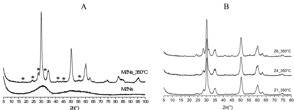
**Figure S1** A) A representative XRPD pattern of the MZNs (Z1) after purification process *via* vacuum extraction, and after heating at 350°C. The marked peaks (\*) were related to monoclinic zirconia phase. B) XRPD patterns of different samples after calcination.
