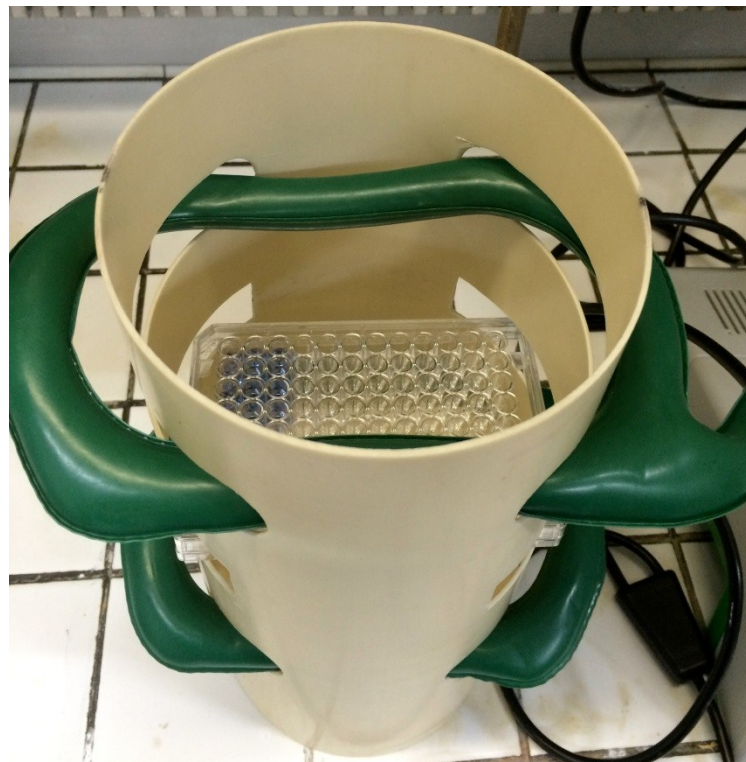
Figure S1. Pictures of the home-made device for the experiments in presence of pulsed electromagnetic fields (PEMF).
