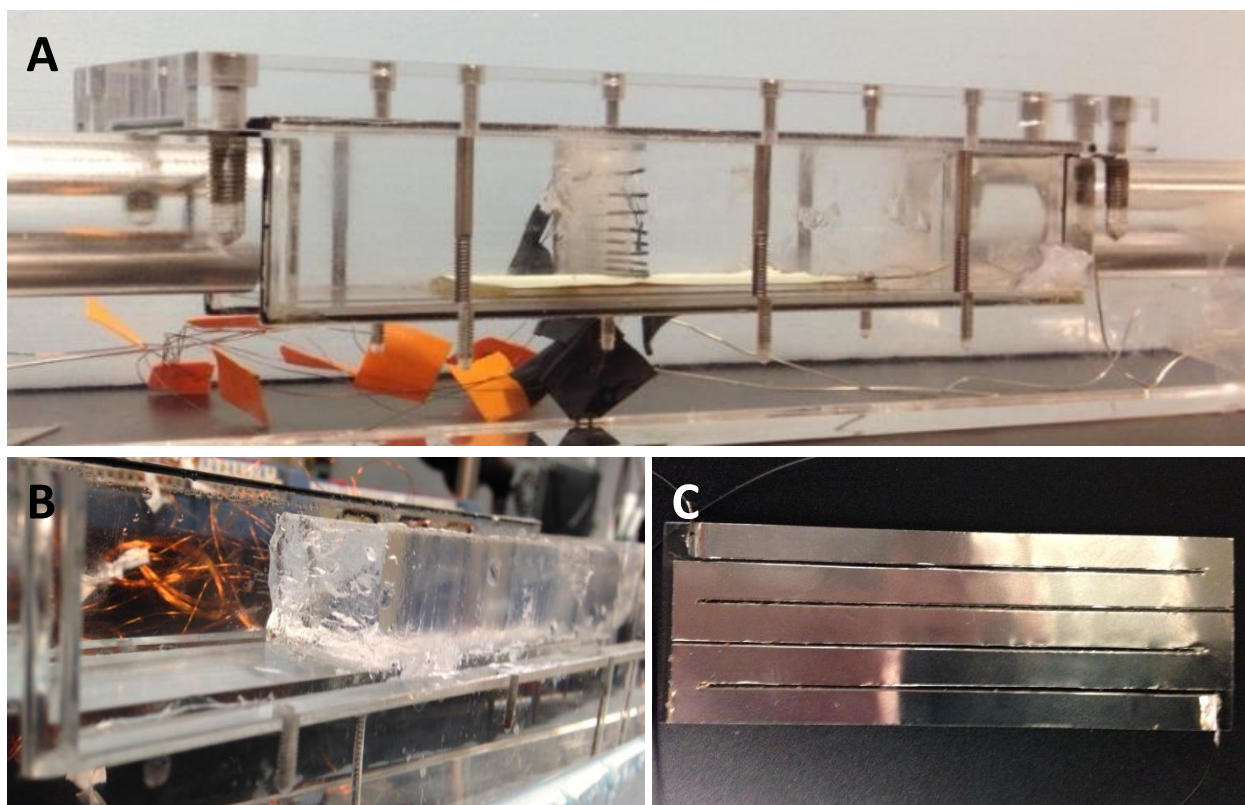
Figure S6. Acrylic chamber used for thermal model (A) 6.45 \text{ cm}^2 cross-section of PVA hydrogel tissue mimic (B) 19.3 \text{ cm}^2 -area, 25 \text{ }\mu\text{m} -thick, nichrome foil heating element (C).
