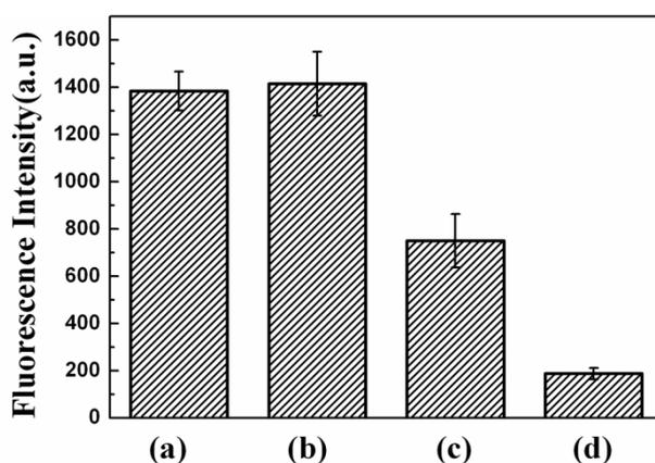
**Figure S1.** Fluorescence Intensity of FITC-Fib absorbed on the surface of (a) virgin PP, (b) Ag NPs absorbed surface of virgin PP, (c) PP-g-P(NIPAAm-co-APMA) and (d) Ag NPs absorbed surface of PP-g-P(NIPAAm-co-APMA)
