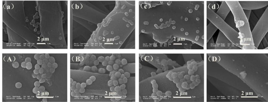
**Figure S3.** SEM images of *S. aureus* adhered on the surface (a-d) and incubated on the surface for 24 h (A-D) of (a and A) virgin PP, (b and B) Ag NPs absorbed surface of virgin PP, (c and C) PP-g-P(NIPAAm-co-APMA) and (d and D) Ag NPs absorbed surface of PP-g-P(NIPAAm-co-APMA).
