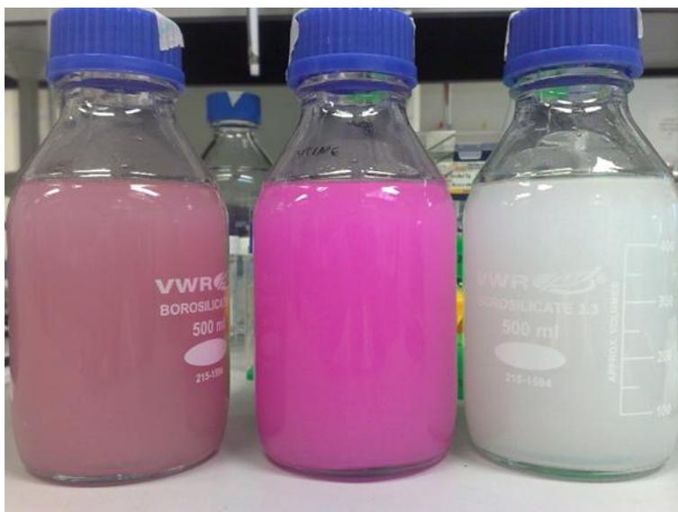
**Figure S1.** Digital images of ZIP highly stable colloidal suspensions in water following 24 hrs of reaction. From left to right: AuNP@ZIP (pink), RhB@ZIP (magenta) and ZIP colloidal particles (white).
