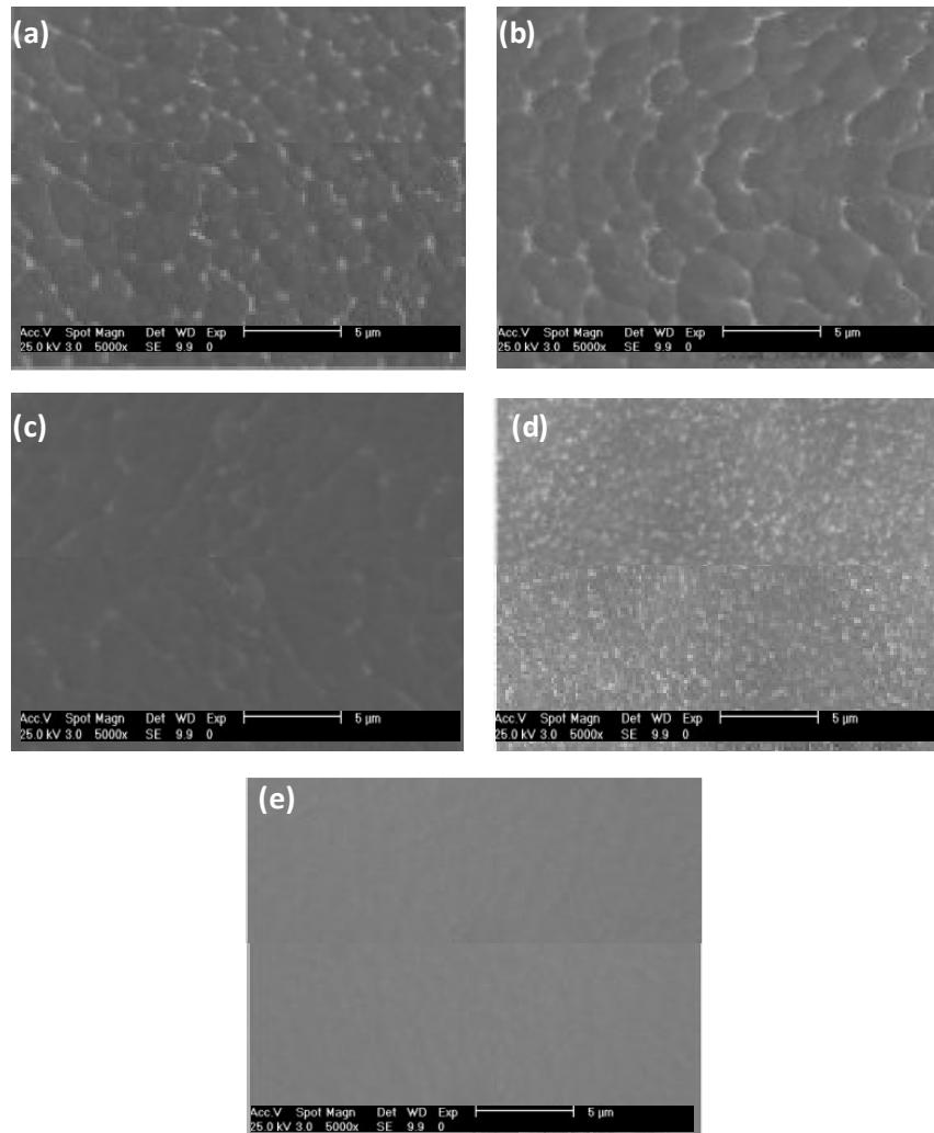
**Fig. S1.** Low magnification SEM images of CS-g-PCL/PHBHHx fibers: (a): 100/0; (b): 70/30; (c) 50/50; (d) 30/70; (e) 0/100.
