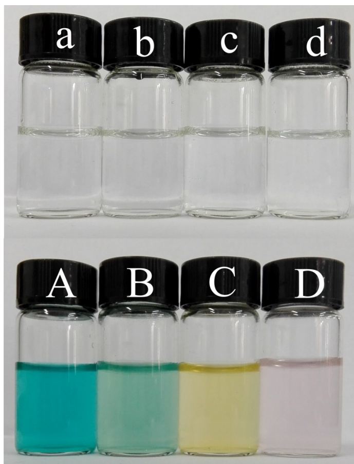
Fig. S7 Images of oxidation color reaction of TMB (a), ABTS (b), OPD (c) and p-hydroxybenzoic acid /4-aminoantipyrine (d) by \text{H}_2\text{O}_2 before (above) and after (below) by the catalysis of MIL-101(Cr)@PB.
