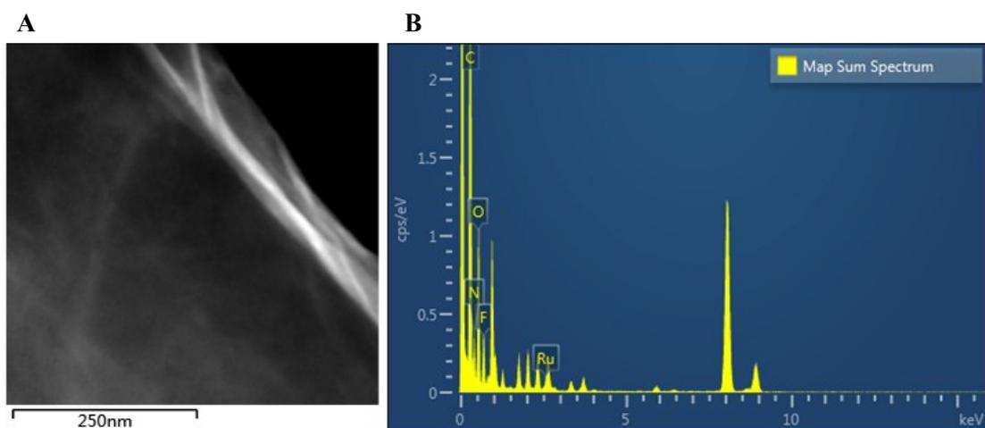
**Fig. S3** Electron images of GO-OMO hybrid (A) and EDS (B).
