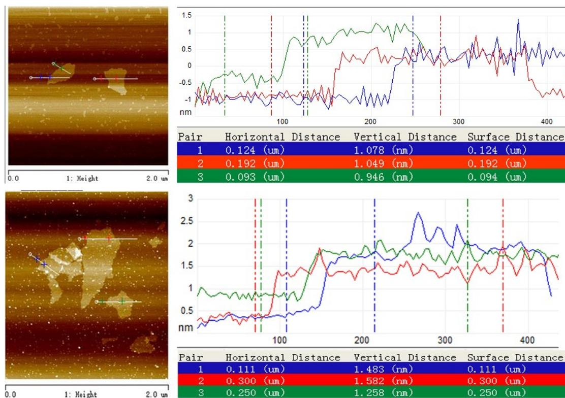
**Fig. S1** The atomic force microscopic (AFM) images of GO (above) and GO-OMO hybrid (below). The average vertical distance of monolayer GO and GO-OMO were 1.02 nm and 1.44 nm, respectively.
