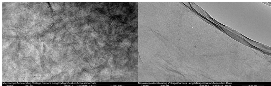
**Fig. S2** TEM images of GO (left) and GO-OMO hybrid (right). The concentration of GO and OMO were 40 μg/ml and 2 μM, respectively.
