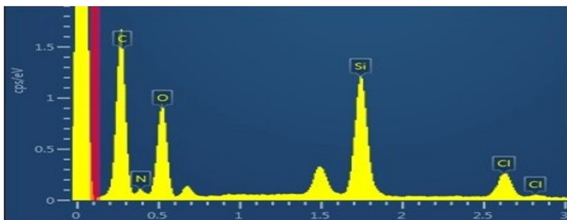
Figure S1: EDX pattern of ONBCbl-SiQDs showing the presence of constituent elements.
