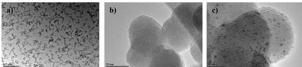
**Fig. S1** TEM images of a) PEGC-FMSNs, b) CTxB-FMSNs and c) negatively-stained (Nano-W) CTxB-FMSNs.
