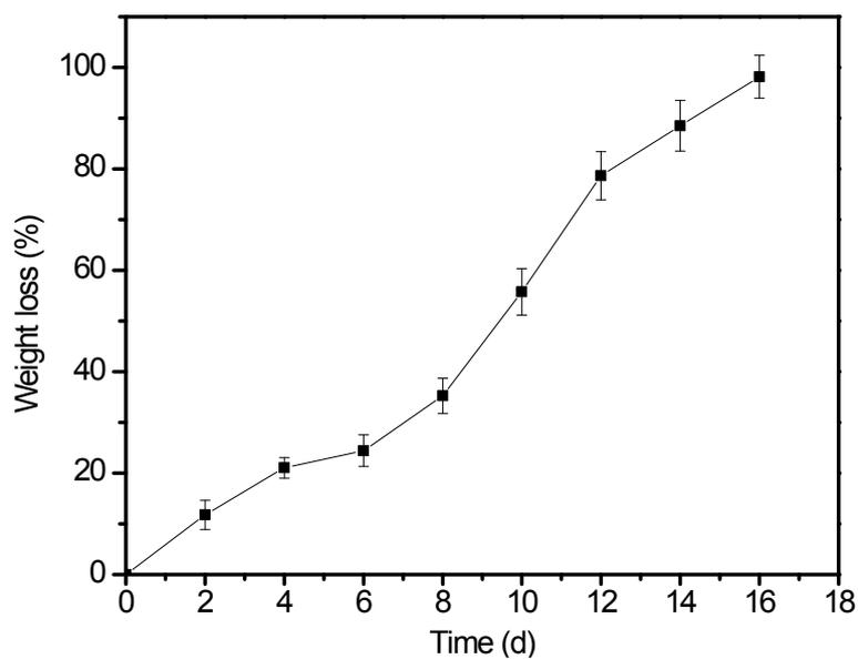
Figure S1. The degradation profile of PUU nanoparticles at 37 °C in enzymatic environment.
