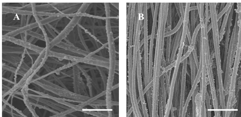
Figure S2. SEM images of (A): random PLA nanofibers/ PLA nanoparticles, and (B): aligned PLA nanofibers/ PLA nanoparticles. Scale bar = 20 μm.
