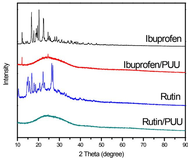
Figure S3. XRD patterns of model drugs and drug-loaded PUU nanoparticles.
