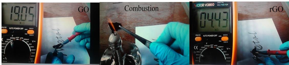
Fig. S5 Resistances of GO films and rGO films observed by a multimeter.
