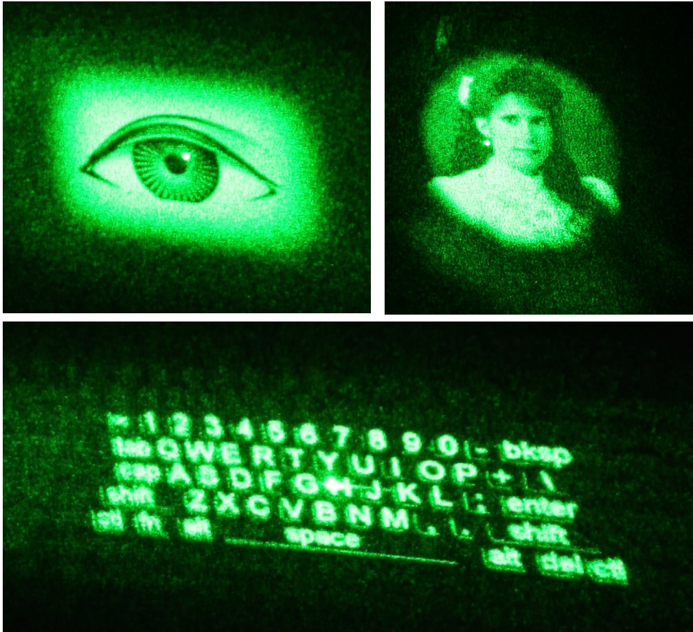
Figure S2. Photograph of projected patterns obtained from propagation of a green light laser source through keratin-made 2D diffractive phase masks. The images are taken at a distance of 10 cm from the keratin optical element. (Master from Digital Optics Inc., Tessera Corporation).
