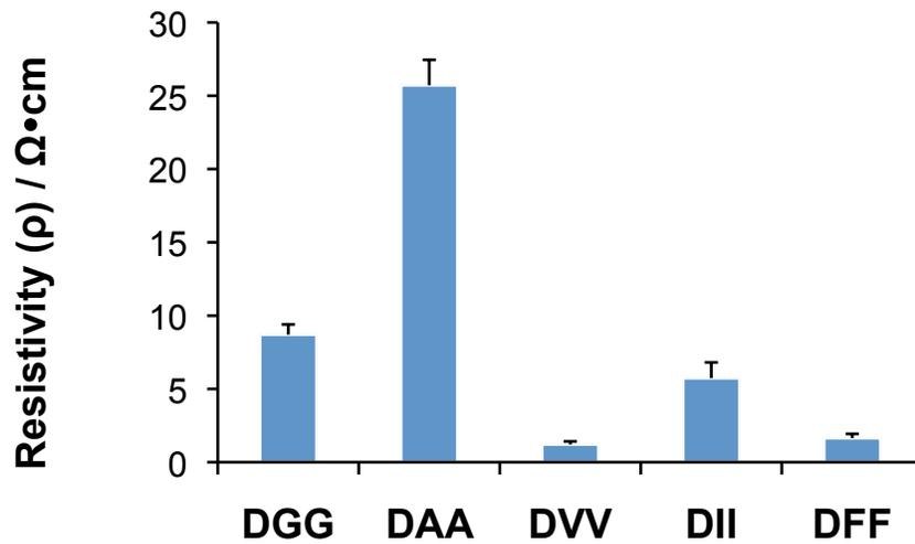
**Figure S32.** Resistivity data ( $R_S \times$  measured mean thickness) for dried, acid-assembled DXX peptide films.
