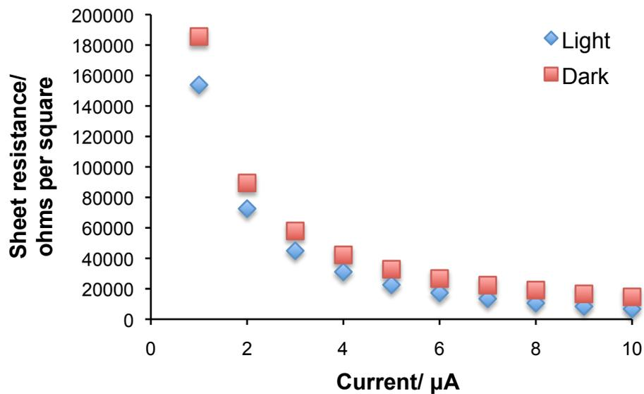
**Figure S35.** Representative sheet resistance vs. current plots for the dried, acid-assembled DGG peptide films under light and dark conditions.
