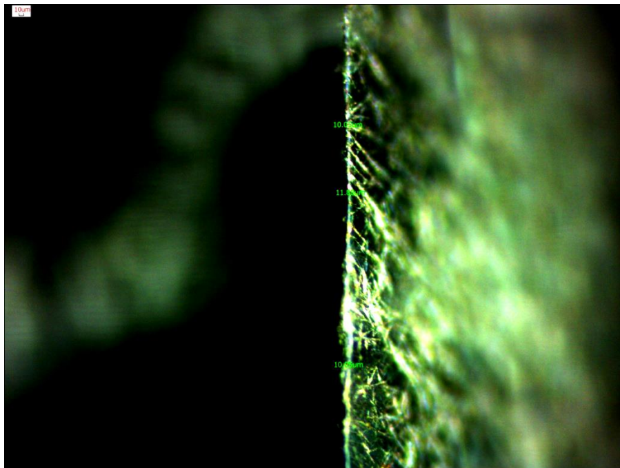
Fig. S2 The cross-section morphology of AgNWs/PI observed by optical microscopy.
